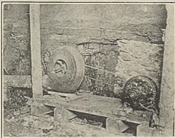
Fig. 17—Blower Fan Ventilating Workings at Anthracite Mine
