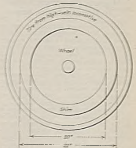
Shim and Tire in Place on Low-Vein Wheel
