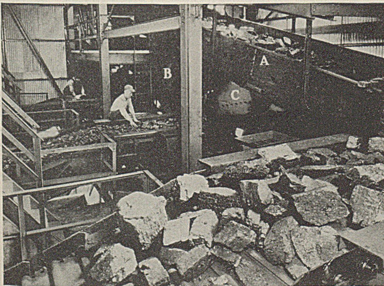
The Screen Section B Operates at Higher Speed Than the Section A-C
