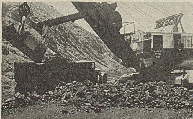
Fig. 5—Loading Coal at Tiger No. 2. This Loading Unit Is Equipped With a 50-Cu.Yd. Aluminum Dipper.
