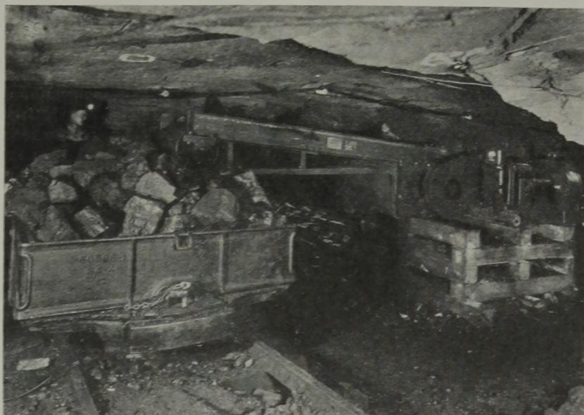
Belt Conveyor Loading a New Car With One-Piece Cast-Steel Body.
