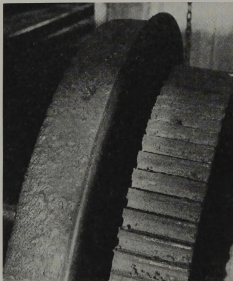
Electrode-Filled "20-Ton" Tire Ready to Be Finished in the Lathe.
