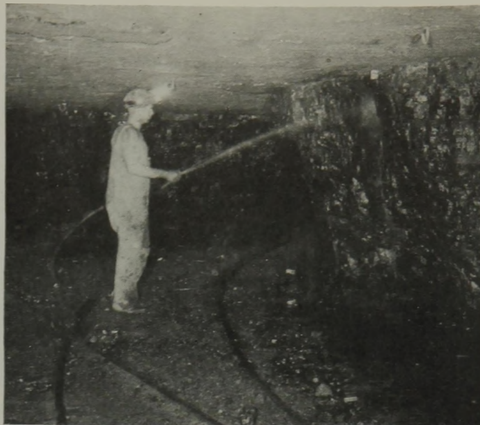
Ribs in Working Sections Are Washed Down to Remove Dust and Clear the Air.
