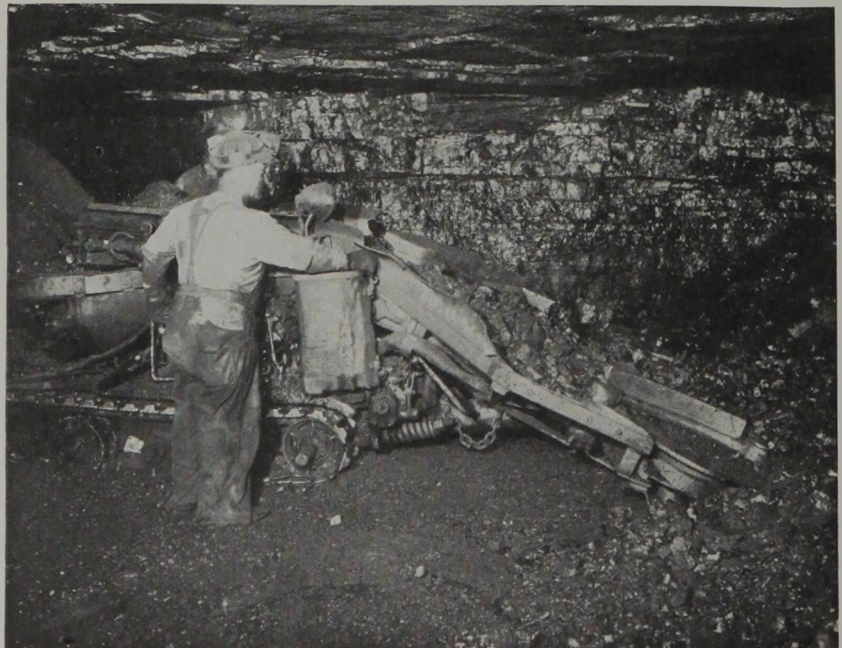
Entries at Kathleen Are Driven by Joy Loaders. This Machine Is Starting a Fresh Cut in a Room Neck.
