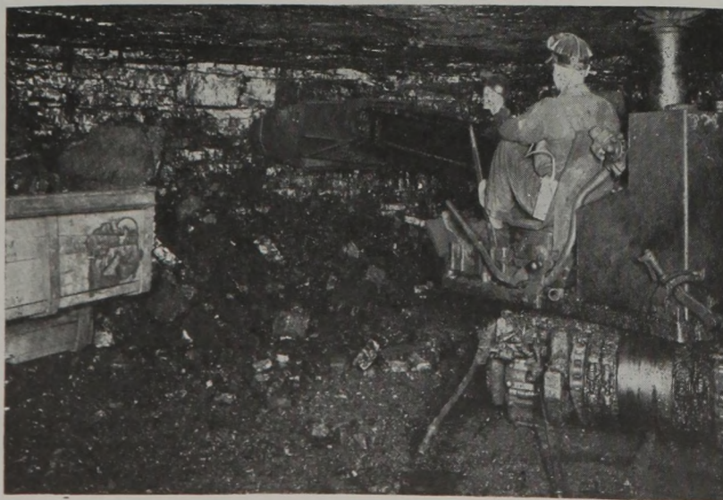
Coal in the Left-Hand Corner Being Loaded by a Goodman Power Shovel to Complete Work in a 26-Ft. Room.
