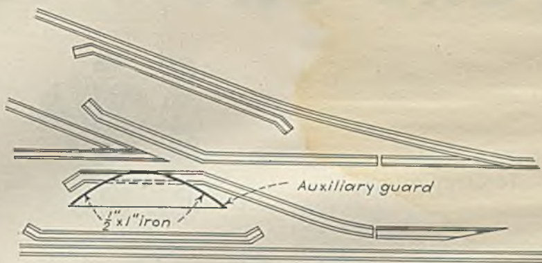
Auxiliary guard in place on frog
