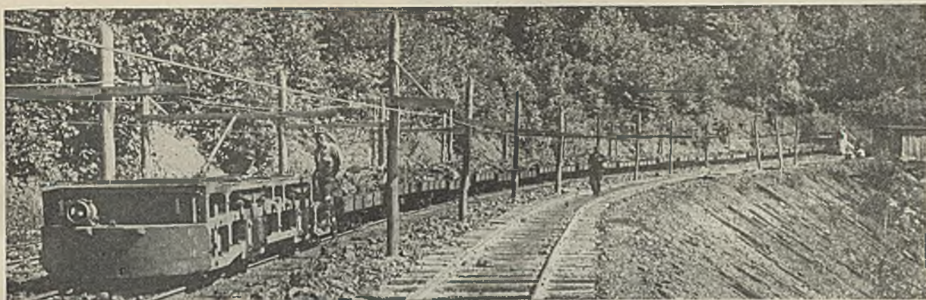
15-ton locomotive with trip on 6,000-ft. outside tram road to Bergoo No. 2 headhouse
