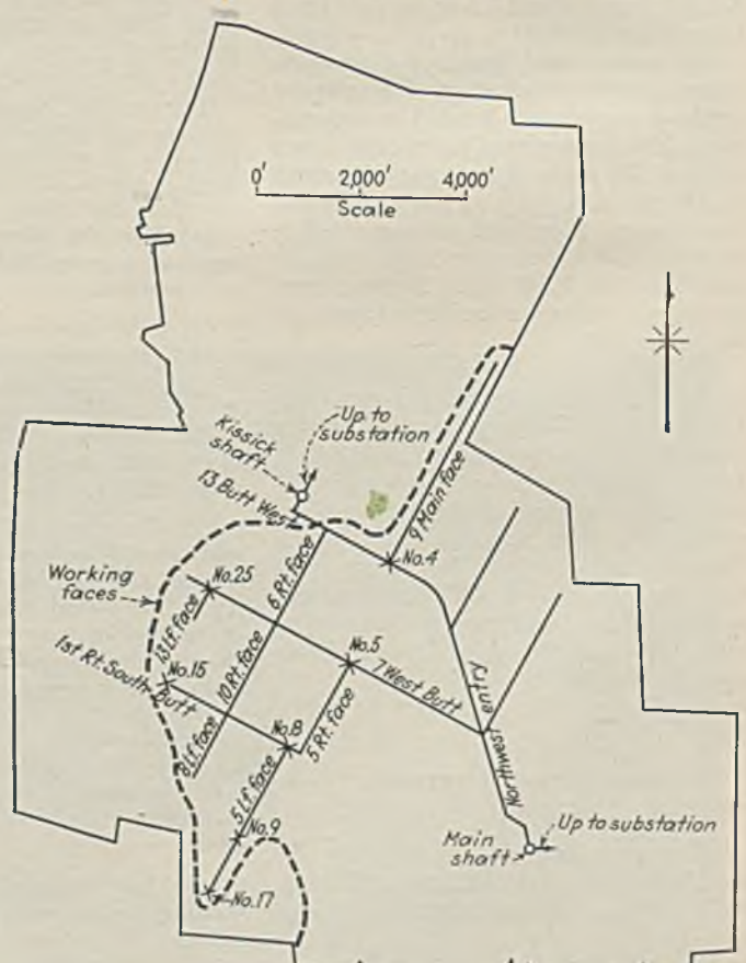
Fig. 2—Distribution system and working faces after completion of second step in improvement program
