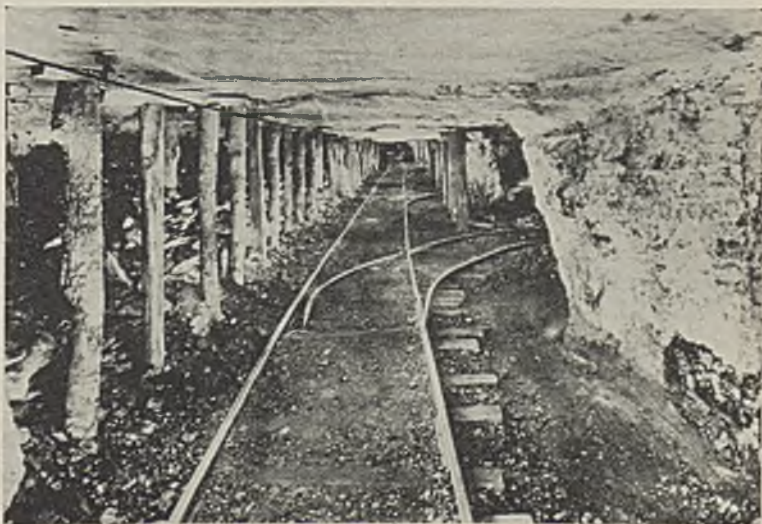
Wide room entry, Alexander mine, with gob placed on side opposite room necks
