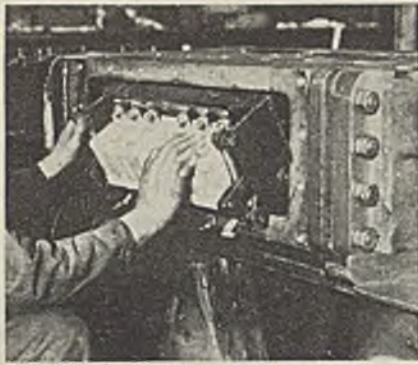
Sullivan "Frigid-Arc" controller on cutter
