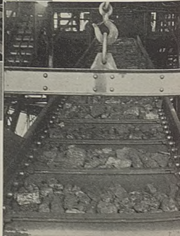
Loading booms are of the flight-scraper equipped with rescreens. The hot-vapor spraying equipment had not been made when the photograph was made
