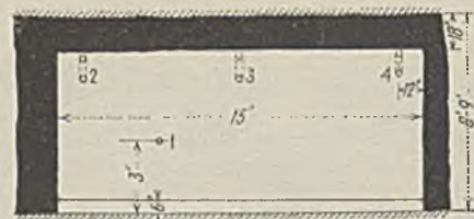
Fig. 3—Hole placement in shortwall places
