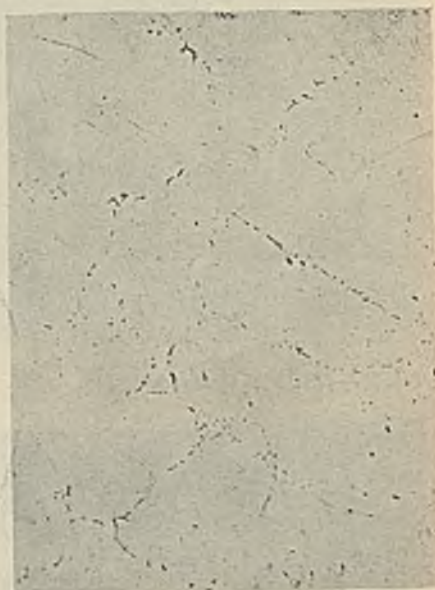
FIG. 15.—AB 3 (2.43 atomic-% Be). Annealed at 810° C. Quenched. \times 100 .
