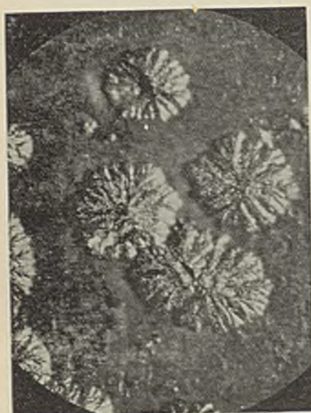
FIG. 7.—Same as Fig. 6. Showing Pits in Zinc.
