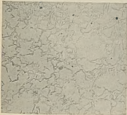
FIG. 7.—42.5 per cent. Palladium. Quenched from 594° C. \times 75.
