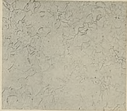
FIG. 6.—40 per cent. Palladium. Quenched from 594° C. \times 150.
