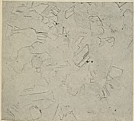
FIG. 9.—45 per cent. Palladium. Quenched from 599° C. \times 150.
