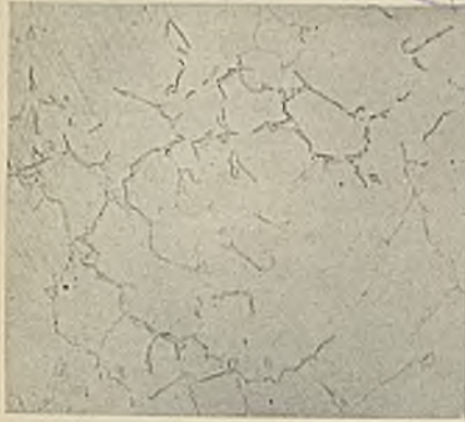
FIG. 5.—40 per cent. Palladium. Quenched from 600° C. \times 150.
