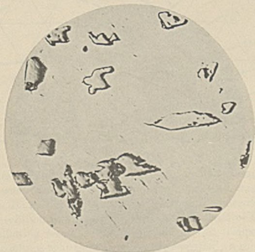
FIG. 6.—Iron 4.34%, Silicon 8.9%. FeSi Crystals. \times 500 .
