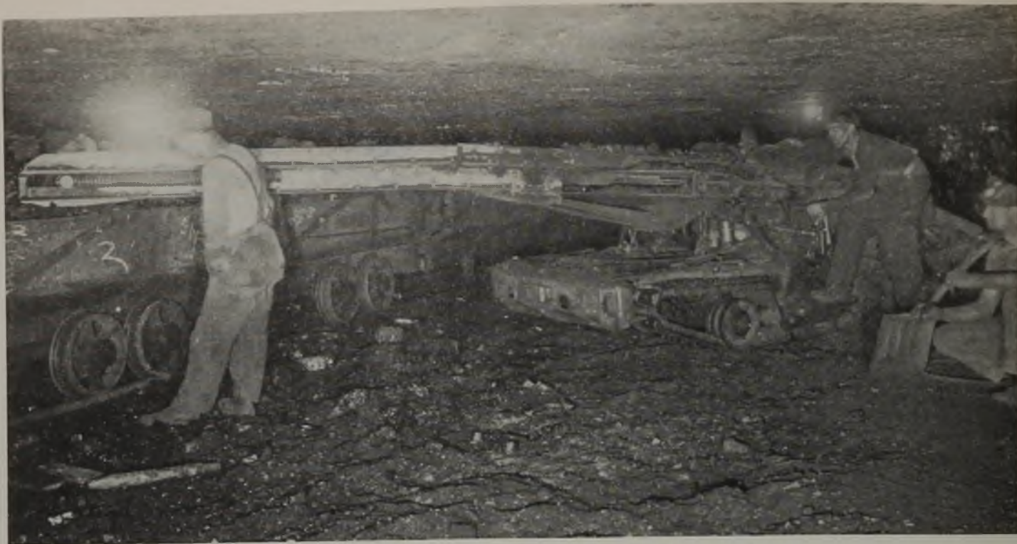
Loading Machine Working Across a 90-Ft. Face in 4-Ft. 9-In. Coal.
