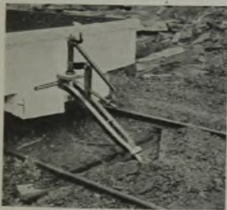
Stopping a Trip. Thrust Members Have Dropped to the Track, Showing Supporting Arm and Pin.
