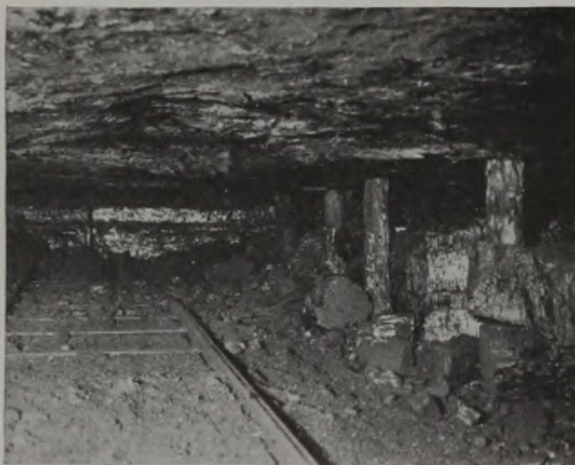
Gobbed on the Right in This Room Are 14-In. Blocks of Bone and Top Coal.
