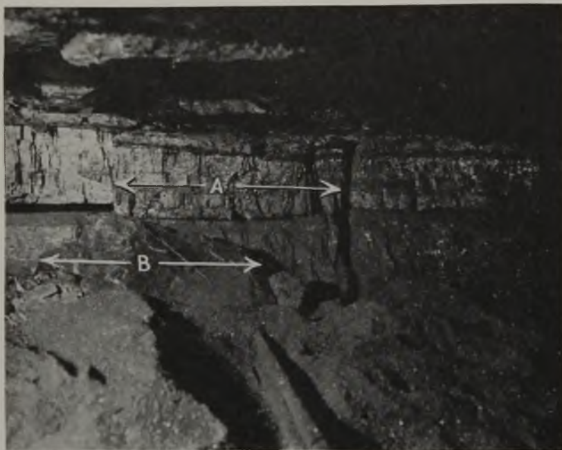
Sawing Has Been Completed. Coal and Bone Above Top Cut Have Broken Down for Length "A" Adjacent to Center Shear Cut. "B" Is Top Rock Fallen From Above "A."
