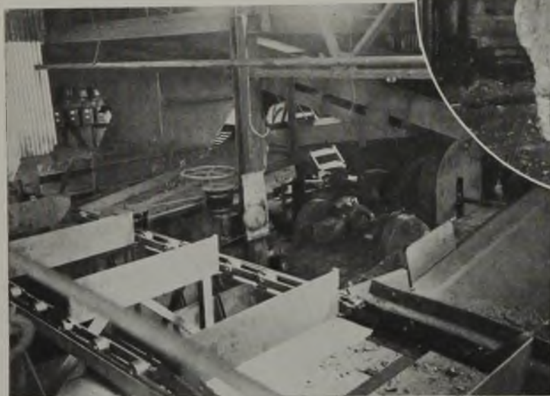
Mine-Run Screens and Shaking Picking Tables in Big Chief Preparation Plant. Surge Bin and Feeder for Screenings Appear at Extreme Left.
