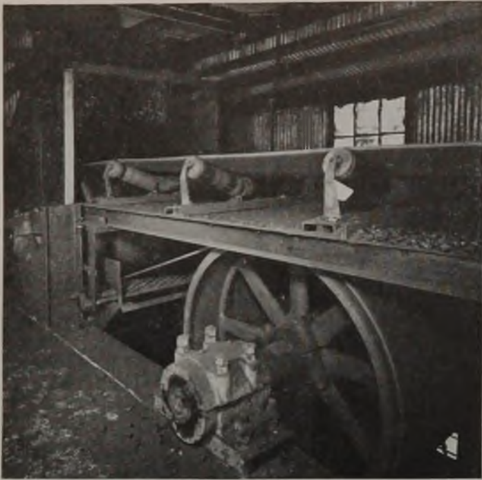
Head pulley, left; rubber cleaning brush, lower center; and upper pulley of tandem drive of slope belt
