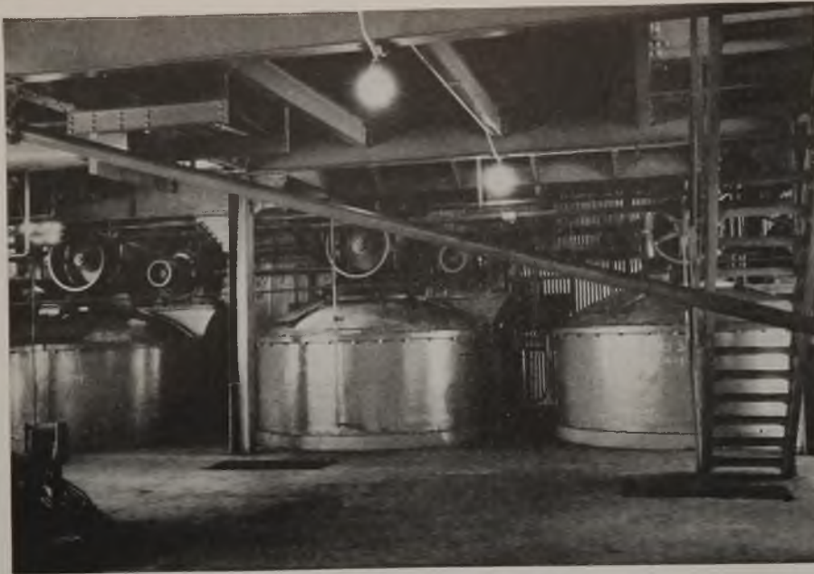
Battery of three Type AR-12 centrifugal dryers
