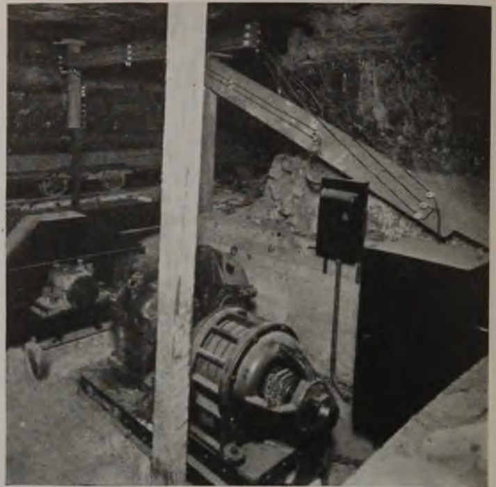
Trip feeder drive at bottom of slope at Van Lear preparation plant in Miller's Creek field of Kentucky
