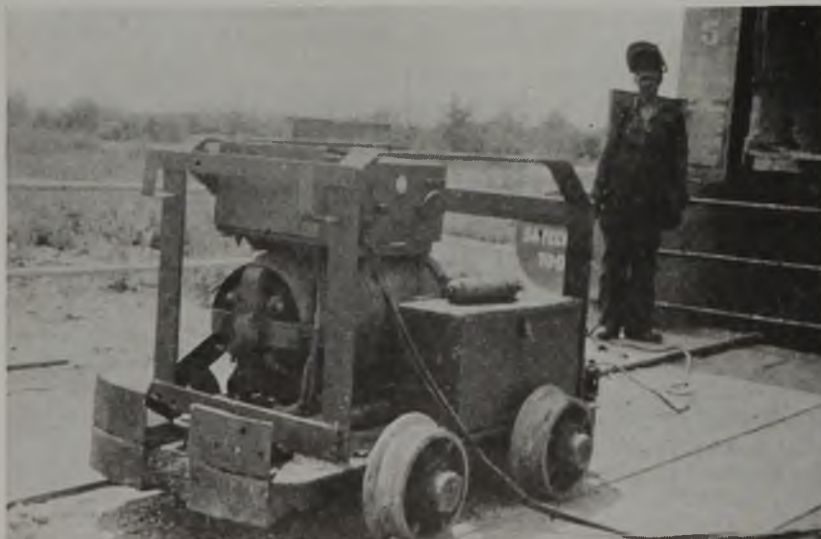
Adaptability to underground as well as surface use features this electric welder
