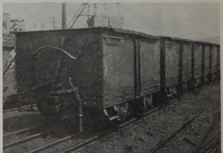
Fig. 12—Lansford car with cast-steel underframe, brakes, special wheels, and roller bearings
