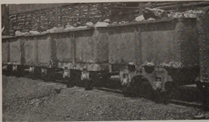
Fig. 10—Cars, right to left, with "bathtub," flat-bottomed with upstanding flange and flat-bottomed cast-steel underframes with pedestals, respectively. View shows reduced depth of side and end plates with the newer underframes
