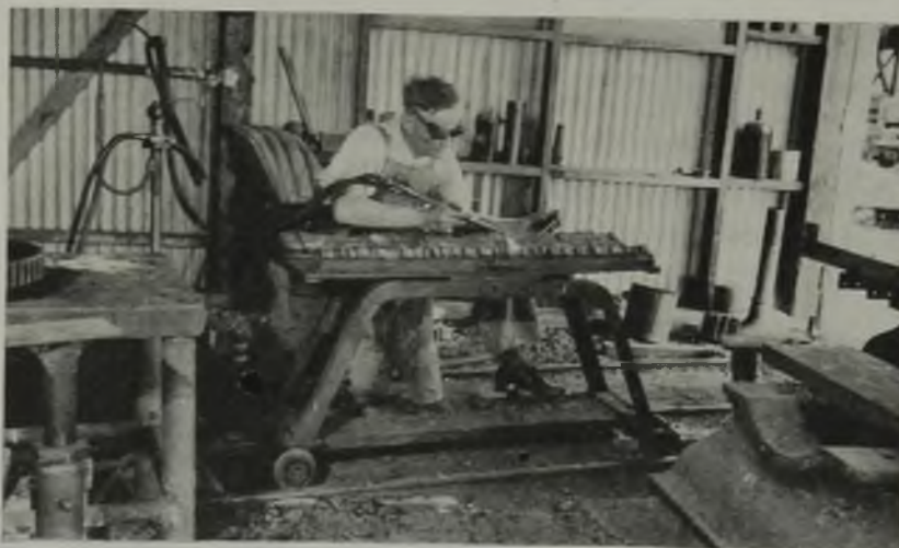
Fig. 1—Two views of the welding jig employed by the author in applying hard-surfacing material
