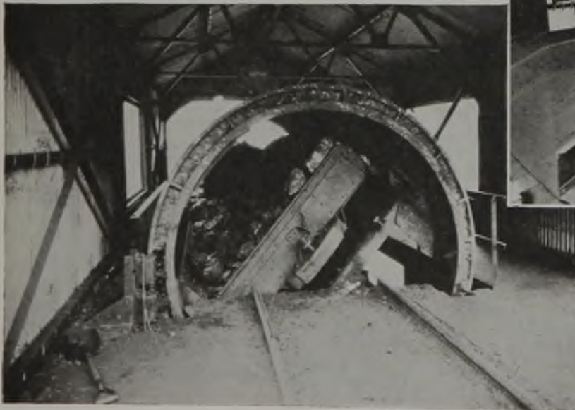
Fingers come out and project over the top edges of the car to hold it as it is carried through a complete revolution
