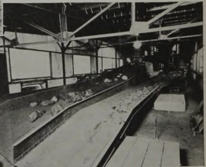
Screening, conveying and display for hand-picking are accomplished by this 20x95-ft. Marcus unit
