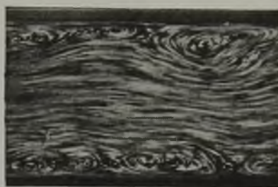
Courtesy United Engineering Trustees, Inc. Fig. 1—Turbulent flow along a straight pipe
