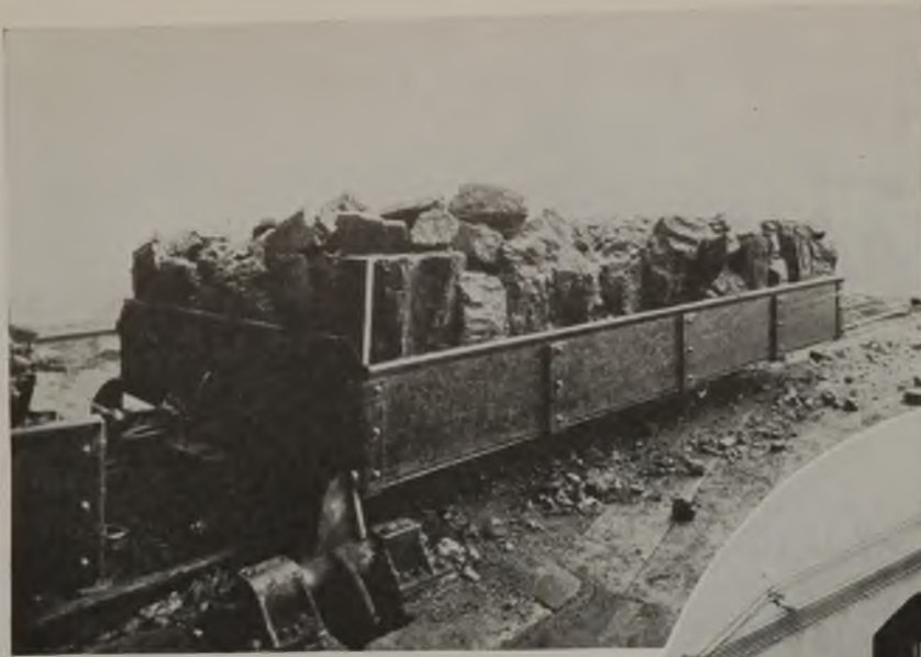
Feeder stops engage the outside corners of car body
