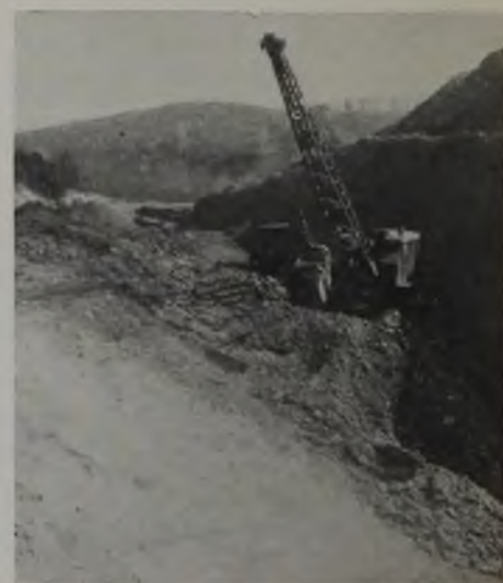
Fig. 7—Dragline loading coal to complete work in Lewis bed stripping, Alliance
