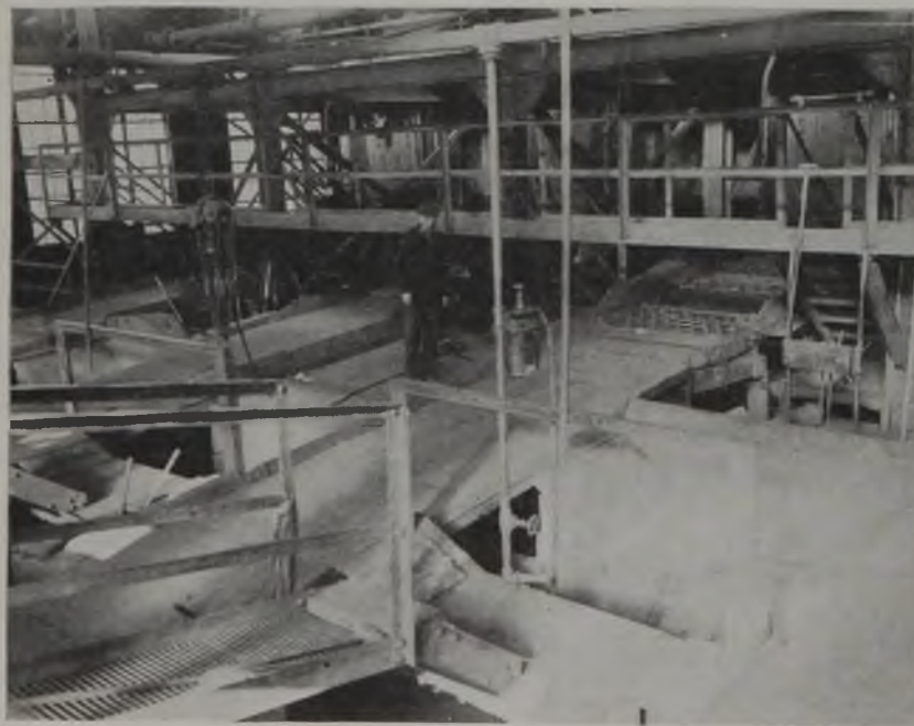
Picking floor, Coaldale breaker. Bull shakers are equipped with cast manganese steel plates to resist wear
