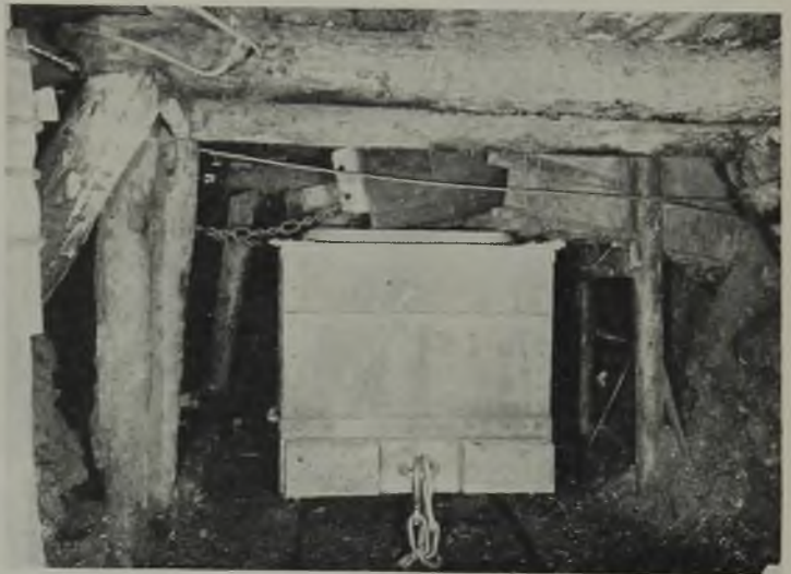
One of seventeen scraper units discharging into car at Cranberry colliery
