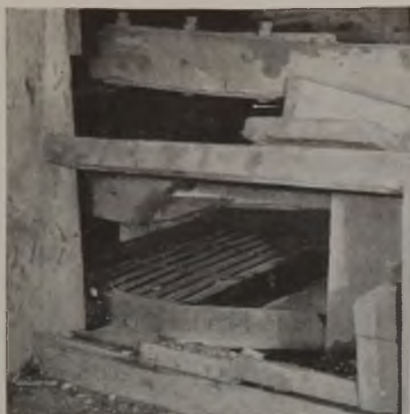
Shutter-type flat picker on end of chestnut shaker, Greenwood breaker
