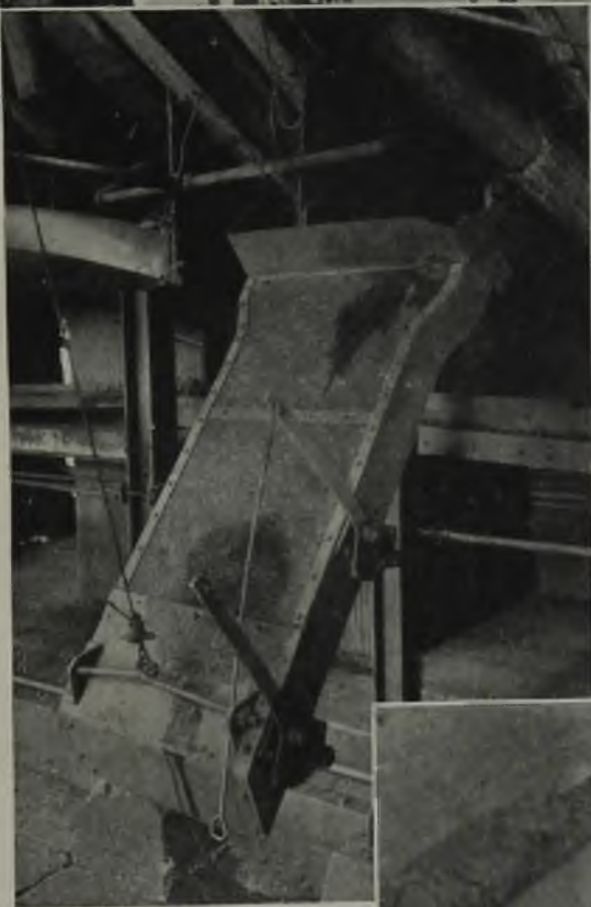
Fig. 5—Coaldale loading chute lowered to working position
