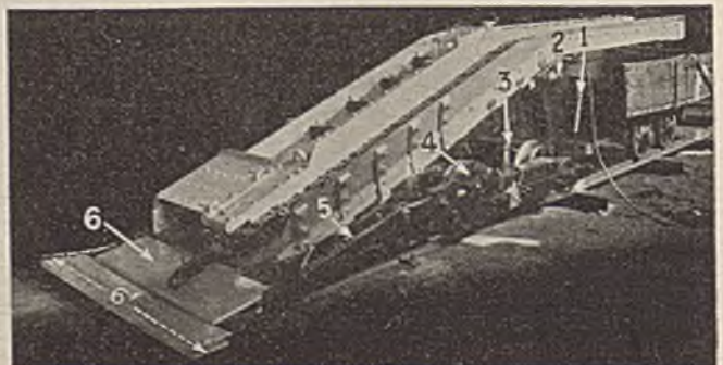
Fig. 3—Left Side of Lang Loader. 1, Brake Lever; 2, Snubber; 3, Tramming Clutch Lever; 4, Feeding Mechanism; 5, Side Arm; 6, Shovel Digger
