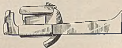
Fig. 3—Hook Embraces End of Girder; Curved Band Engages Post; Wedge and Clamp Hold Two Together
