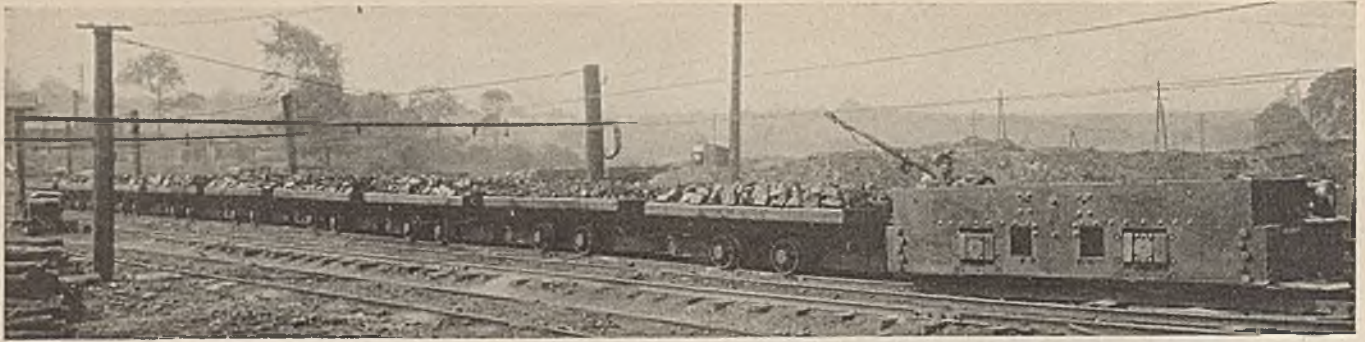
A Standard Trip Consists of Nine 3½-Ton Cars Hauled by a 10-Ton Locomotive
