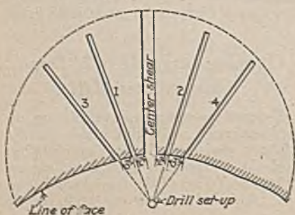
All Four Holes Are Fanned Out From One Central Drill Set-up
