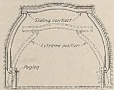
Fig. 1—Curved-Rib Timber Set With Peg-Leg Footing and Sliding Contact Between Post and Cap
