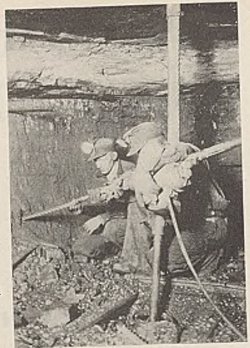
These Two Men Bugdust, Drill, and Shoot Ten Room Cuts in a Shift
