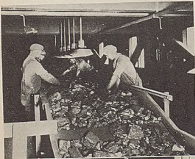
Fig. 1—Flashlight of First Special Picking - Table Lighting System, Cardiff Mines, Imperial Coal Corporation
