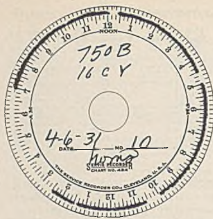
Fig. 3—Recorder for Registering Operating Delays Used on Both Stripping and Loading Shovels; Taken From 16-Yd. Shovel
