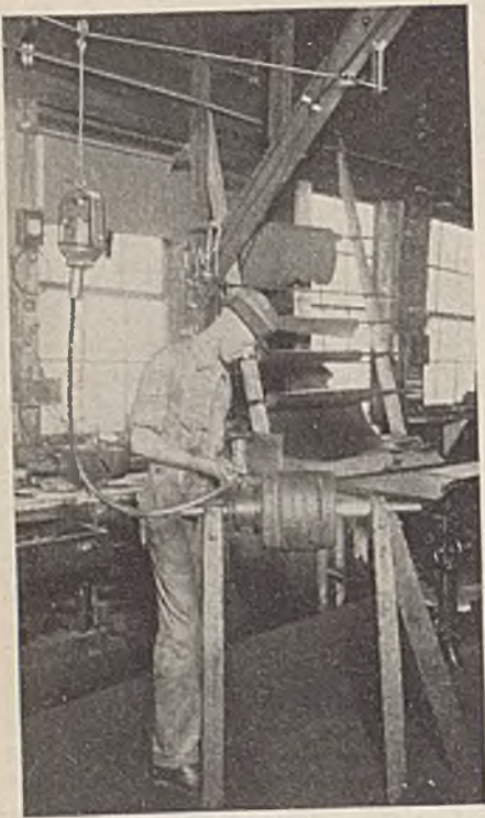
Handy Position for the Motor While Slotting a Commutator
