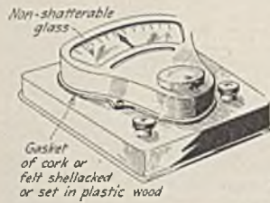
Fig. 2—Keep the Ammeter Dustproof
