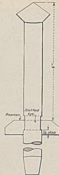
This Tool Drills and Reams in One Operation
