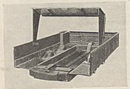
Enterprise Low-Type Mine Car
