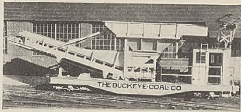
Fig. 5—On Different Sections of Track the Slate Larries Operate From Third Rail, Pantograph, and Trailing Cable
