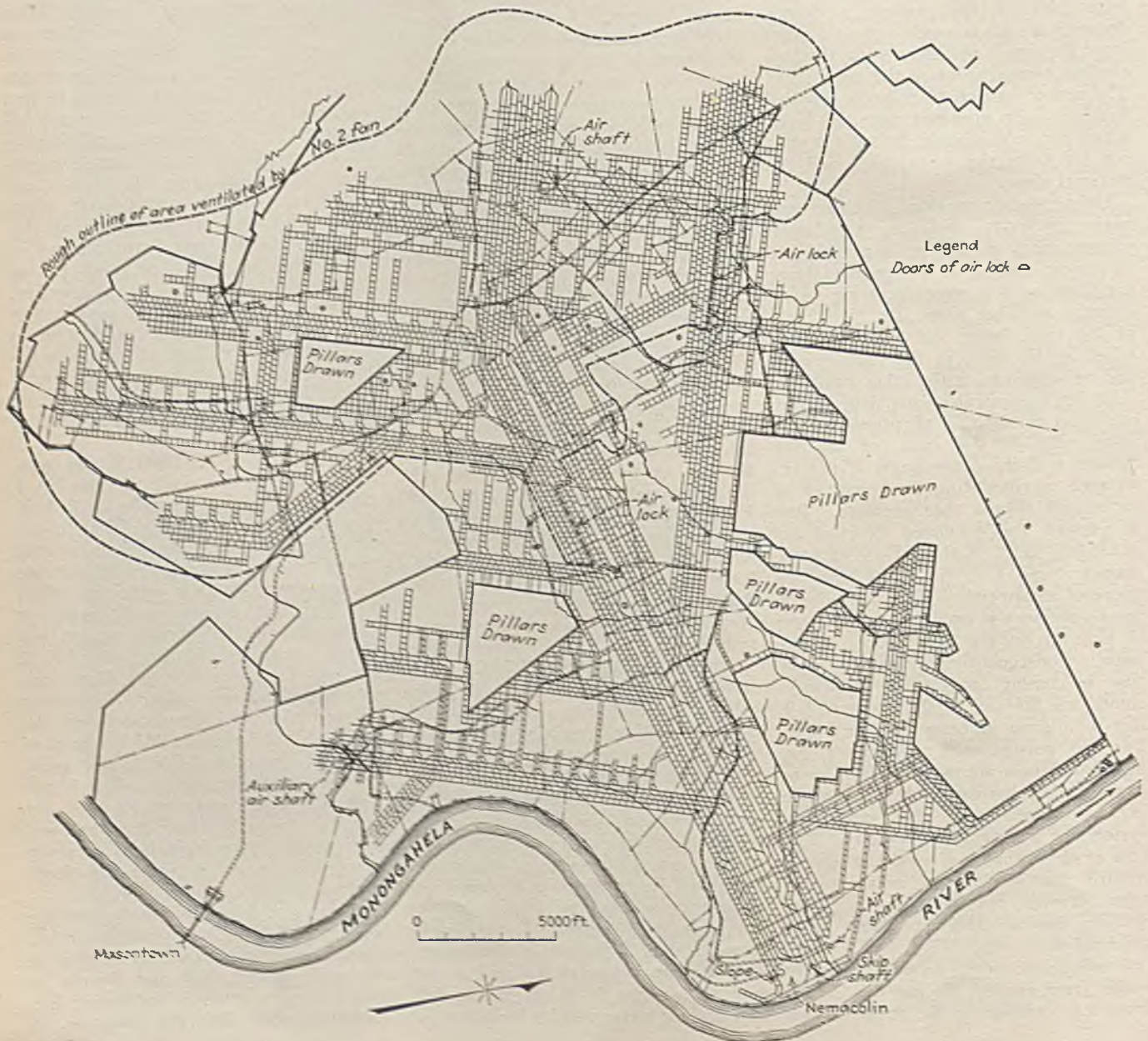
Fig. 1—Nemacolin With Its Intakes, Returns, and Airlocks
