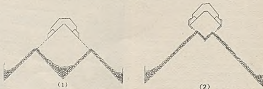
Fig. 3—Sketch Showing Tripper Spouts (1) Without End Plates to Reverse Coal Flow (2) With Such Plates. Also Piles in Bin Without and With End Plates
