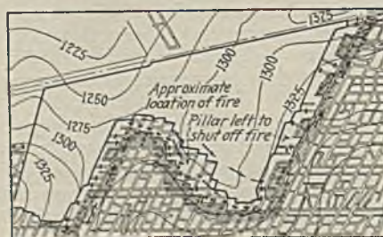
Fire Occurred Where a Salient Angle Caused Pressure and Grades Induced Standing Water
