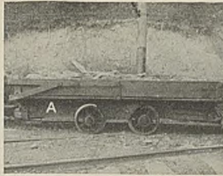
Fig. 4—Old Car With Bumpers Sagged Close to Rail
