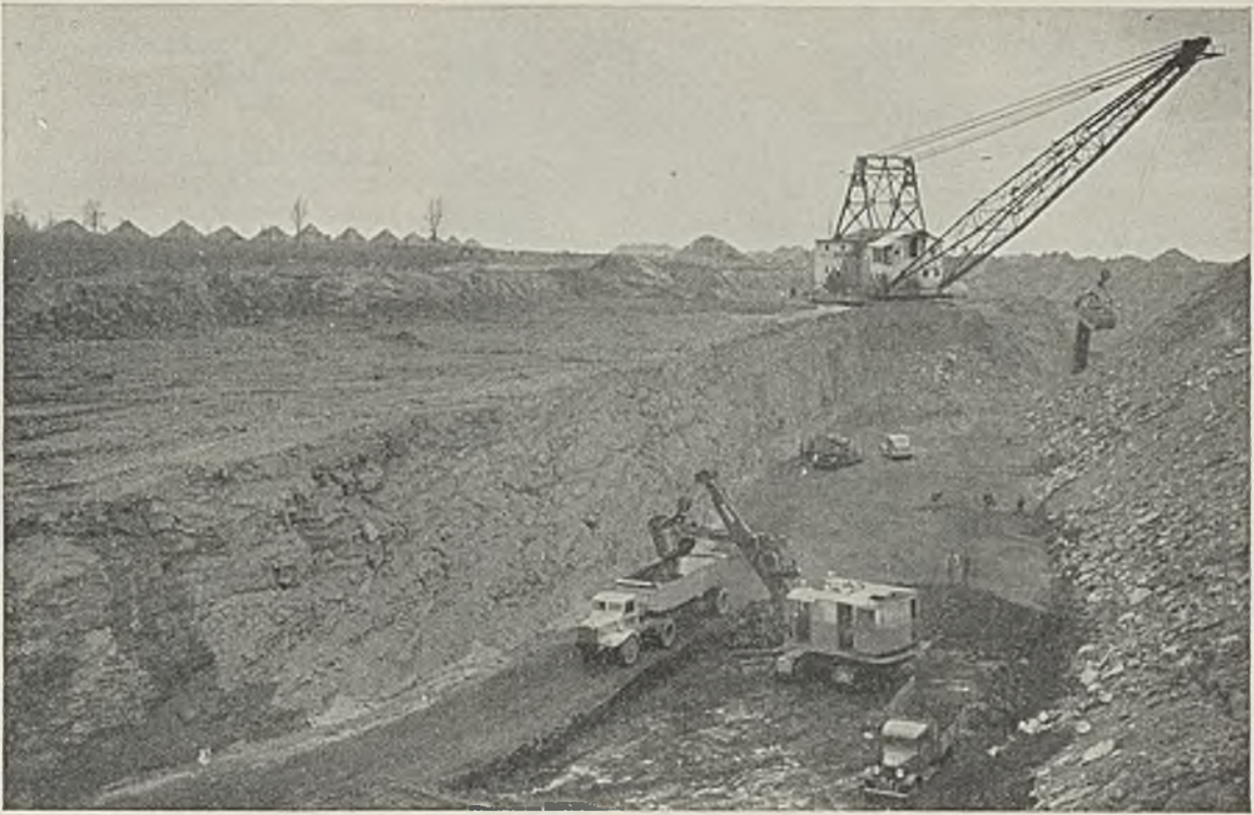
General view of the Old Glory pit, showing how the dragline works from a bench made by taking the clay off down to the gray slate
