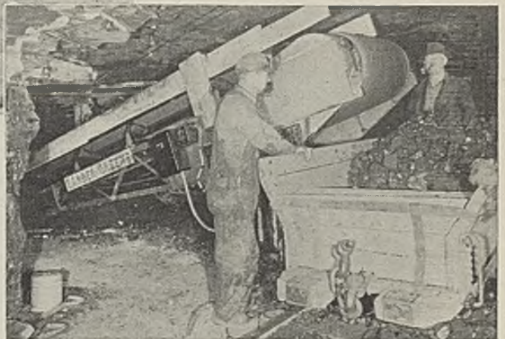
A 54-ft. belt conveyor with push- button control brings coal up from the dump hopper to the trip loading station. In the rear is C. C. ("Daddy") Wilson general superin- tendent, who opened No. 2 mine
