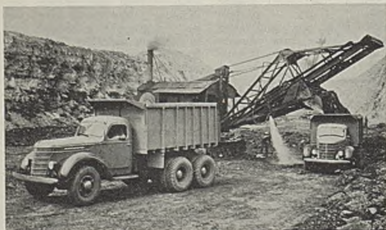
Ten-ton end-dump trucks are used for transportation by the Crowe Coal Co.
