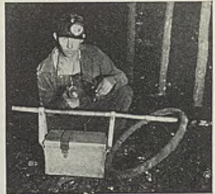
Earphones, power box and loop antenna weigh but 25 lb.
