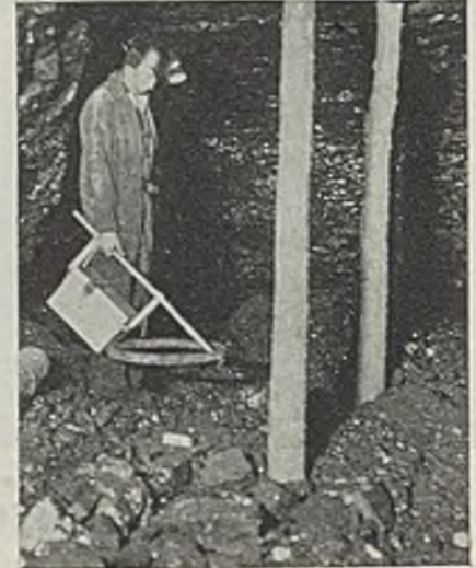
The "bloodhound" has indicated to the hunter that a shell or other metal object is buried in the refuse near the pile of props.
