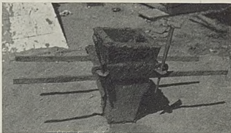
Box which cleans and lubricates the ropes at Zeigler No. 2 mine.
