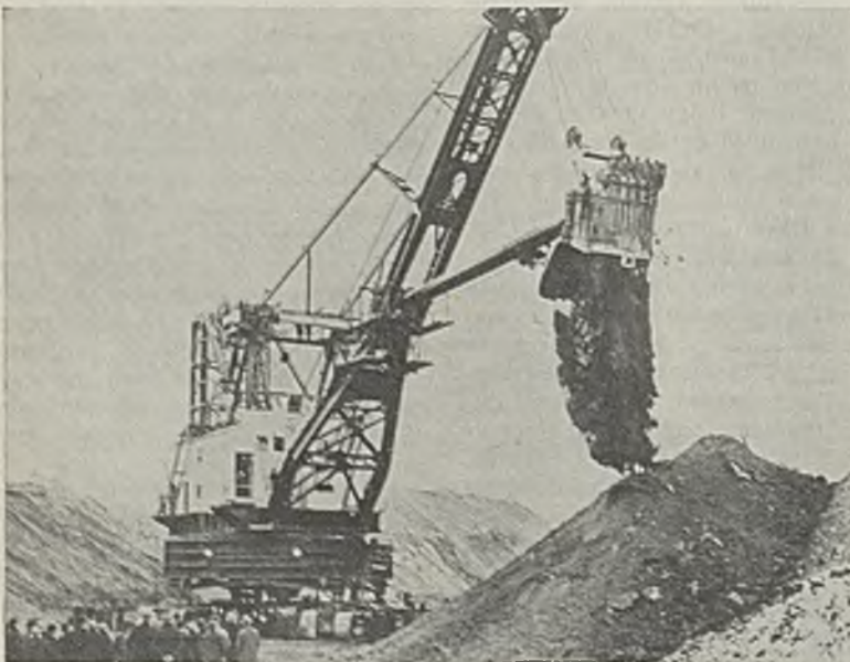
1937 — Overburden at the new Buckheart mine is removed by 30-cu.yd. dipper
