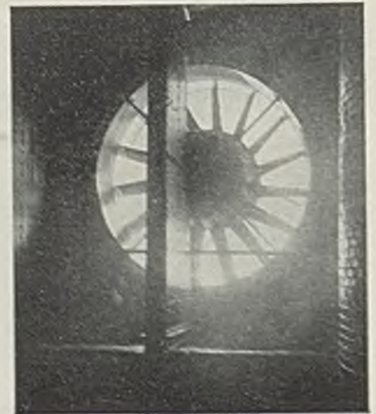
Steel doors folded to the open position in the adapter of the Jenkinjones fan
