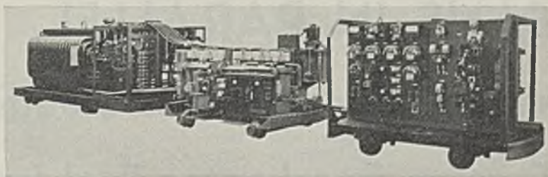
Fig. 6—Shop view of portable rectifier station for the Weirton Coal Co.
