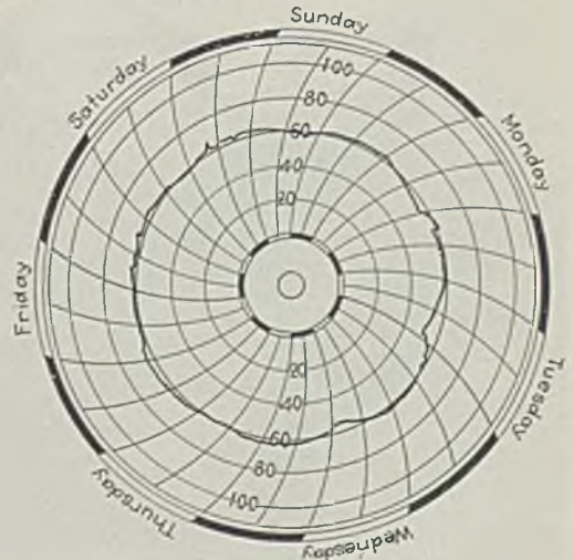
Fig. 3—Temperature record, air entering the shaft, Talleydale mine, July 26 to Aug. 1, 1937, inclusive, with maximum and minimum day-time outside-air temperatures over the same period
