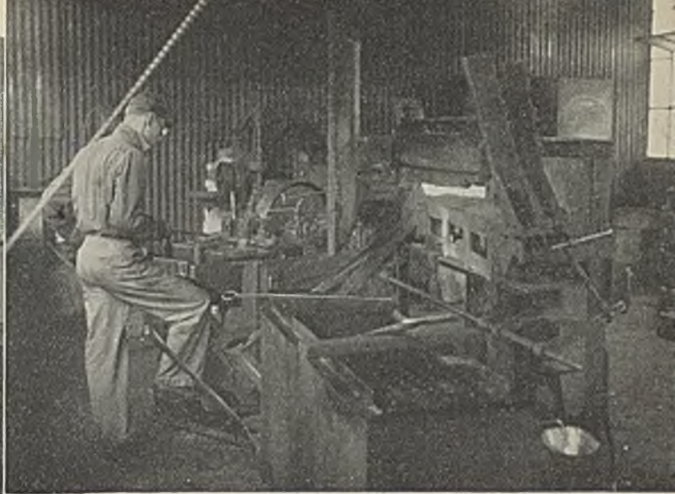
Centralization of bit sharpening at Mount Hope leaves room for mine-car repair work at the mines
