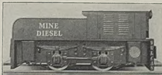
Mine Diesel Locomotives 4 to 12 tons weight, 30 to 100 HP. Built to suit special mine operating and haulage conditions.
