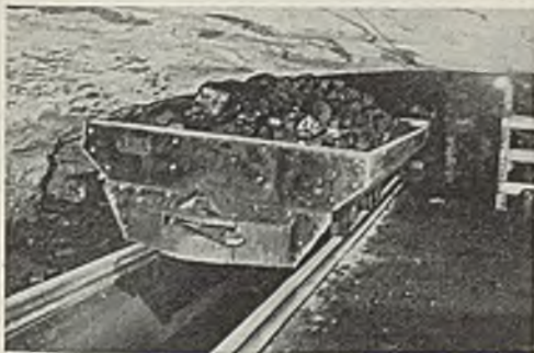
S-D 1-2-3 large capacity cars in the WASSON Mine about to be unloaded automatically.
