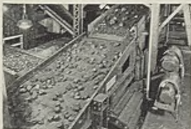
The chute has a slight slope and acts as a feeder. Available in single and multi-deck designs.
