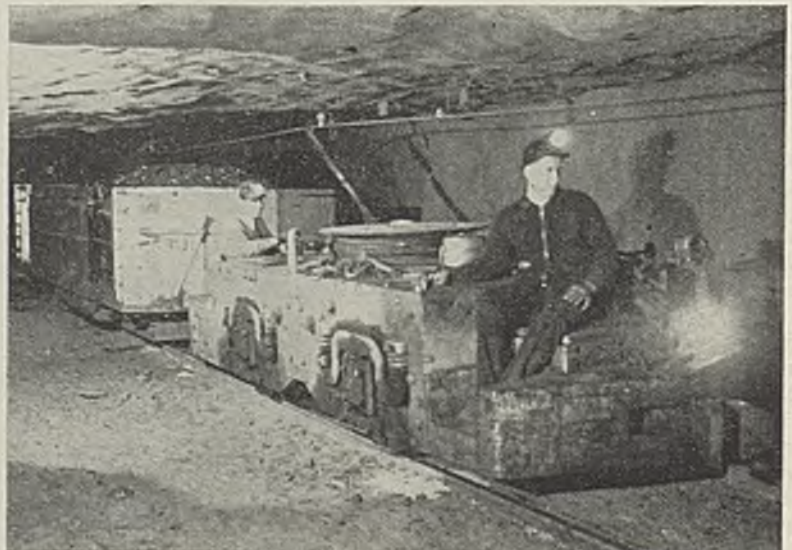
Side view of Isabella gathering locomotive (in extra service on the bottom), showing snapper's quarters.
