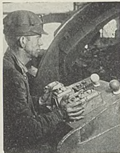
The dumper has the red signal, indicating the car is spotted in the dump, and with his thumbs on the buttons is ready to start the dump the instant the green light indicates that the weigh basket has started to close
