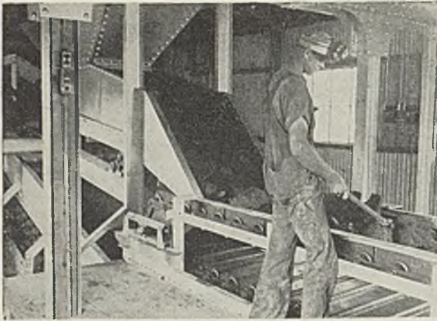
Individual cars of coal selected at random are diverted over the inspection table.
