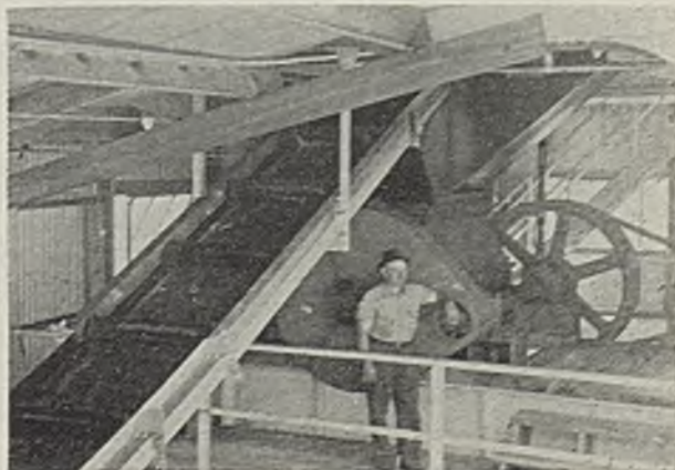
Left—Alternate long and short projecting arms attached to the main shaker at the upper end tip the large blocks of coal so that fines cannot ride them over the screen. Right—A cross conveyor at the ends of the boom encircles the 36x54-in. crusher.
