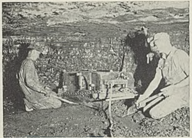
The coal is 3 1/2 to 6 ft. thick and is without regular parting at Blue Heron mine.
