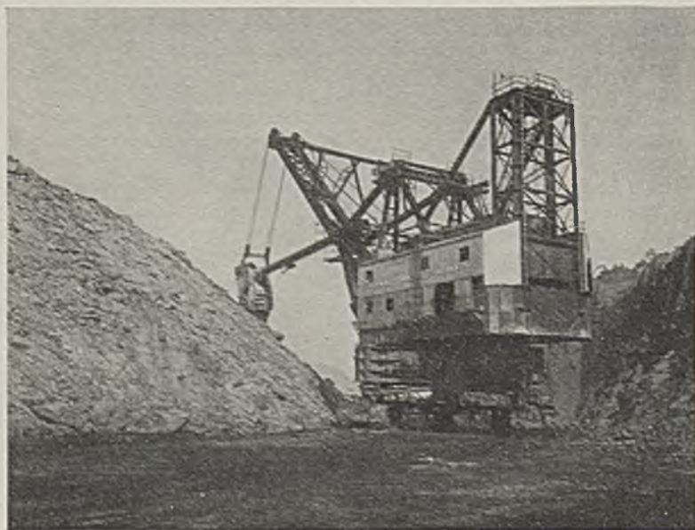
This Bobolink stripping unit is equipped with a 30-cu.yd. welded alloy-steel dipper with counterweight.
