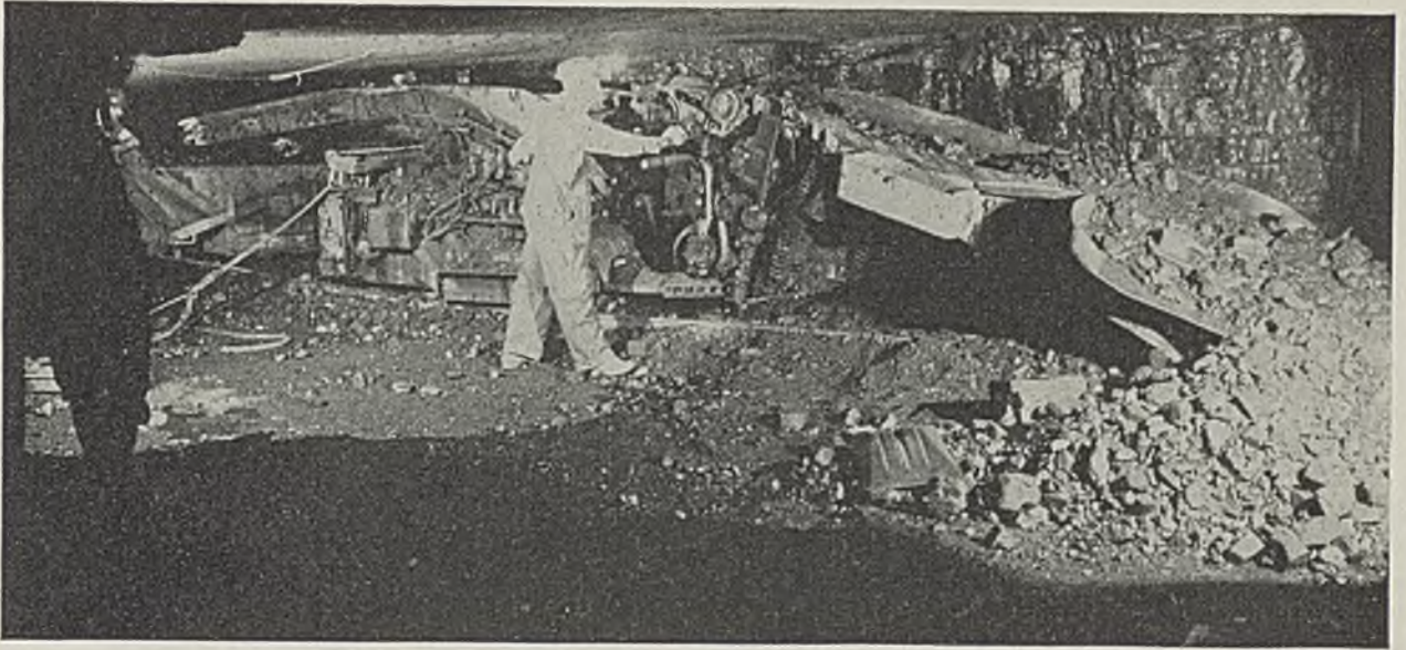
Track-mounted loading machine at work in the No. 6 seam, New Hope mine.
