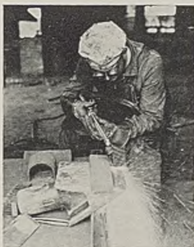
Cutting the dull end off a dipper point at Minnehaha.
