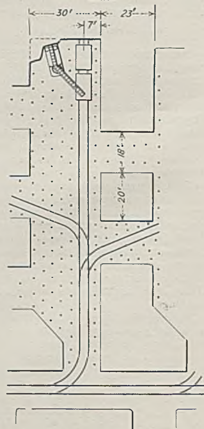
Fig. 23—Diagrammatic sketch of two-car changing system, Knox Consolidated mines
