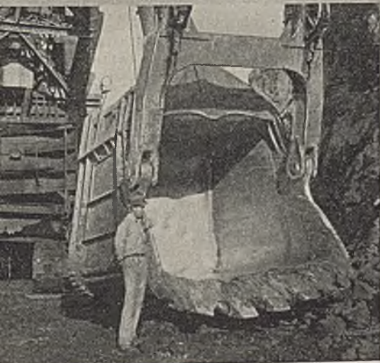
30 cu. yd. all-welded MAN-TEN dipper. Used on 950-B Bucyrus-Erie stripping shovel at the Seeleyville Mine of the Binkley Co. of Indiana. Shovel has 105 ft. boom and 72 ft. dipper handle—52 men can stand inside this giant dipper without crowding.
