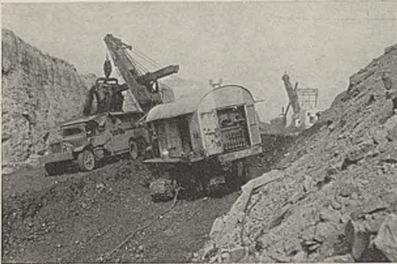
30-ton truck unit at Sunlight receives its load. Note pitch of coal.
