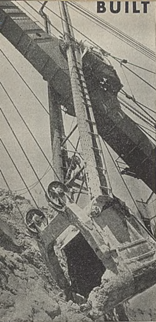
41.6% increase in capacity here. 17 cu. yd. MAN-TEN dipper by replacing a 12 cu. yd. dipper on this 750-B Bucyrus-Erie electric stripping shovel in Friar Tuck Mine, makes it possible to remove 7000 extra cu. yd. of over-burden every 24 hours—with no increase in power equipment.
