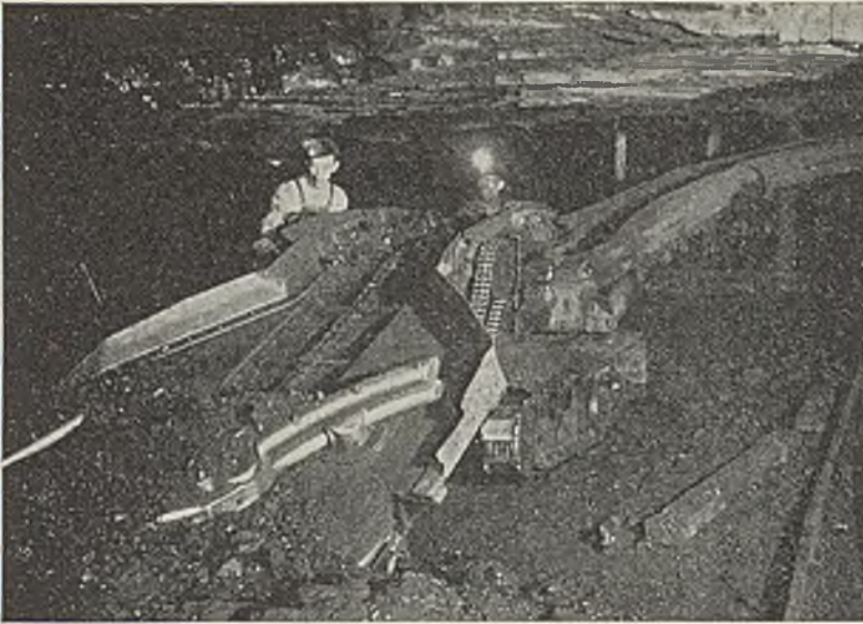
Loader improvements include flat hopper, new drive on front end, springs on swing-jack ropes, etc.
