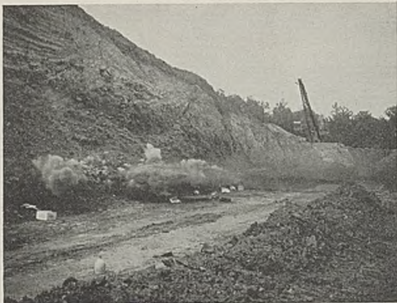
Shooting at Mariah Hill Super Block, with the 5-yd. walking dragline in the background.
