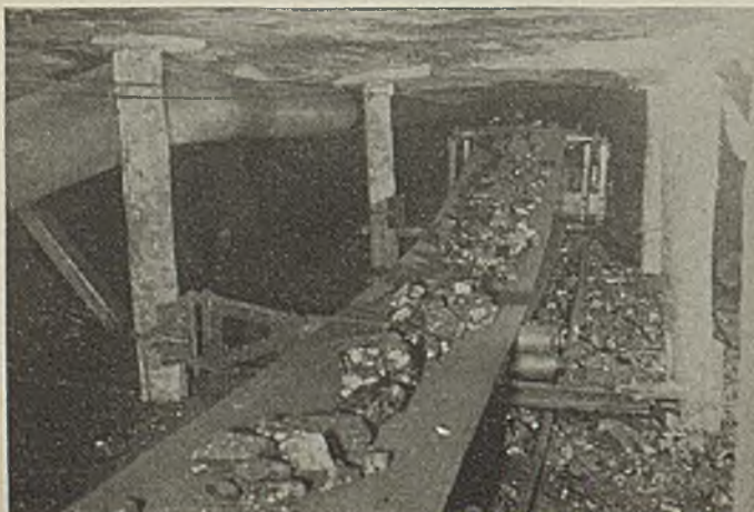
At the Delivery End the Coal Rides Over the Top of the Machine
