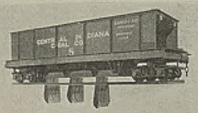
Fig. 12—S & D Large-Capacity Bottom Dumping Car for Stripping
