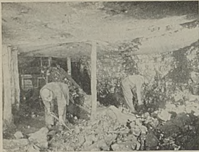
Another View of Conveyor Robbing Pillars in Franco No. 2 Mine
