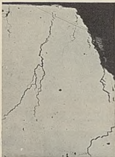
FIG. 6.—Intercrystalline Cracks in Tinned Area Section from Tube A. \times 40
