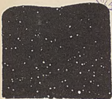
FIG. 3.—Ingot 346 ("3L11"). Solidified under Atmospheric Pressure.
