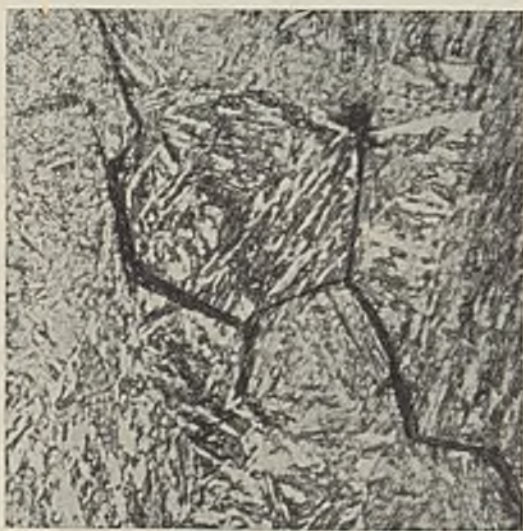
FIG. 8.—Coarse Structure of Tube A and Intercrystalline Cracks (at \gamma Boundaries). \times 800 .
