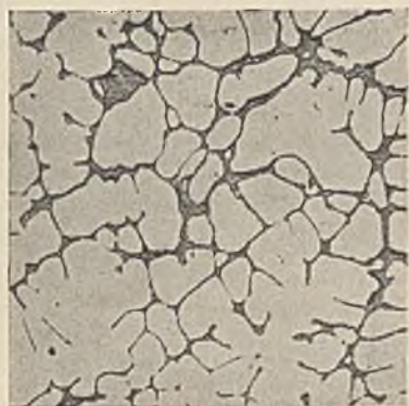
FIG. 10.—Ingot No. 361. "3L11" Alloy Solidified in a Sand Mould under 700 lb./in. 2 Pressure. × 50.
