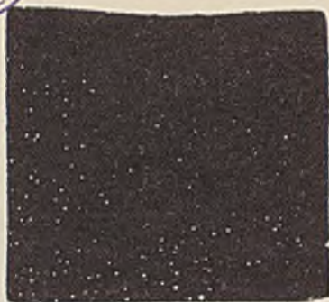
FIG. 4.—Ingot 350 ("3L11"). Solidified under 25 lb./in. 2 Pressure.
