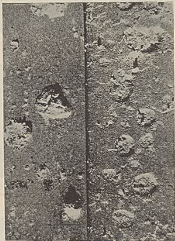
FIG. 9.—Blisters on "3L11" Alloy Solidified in a Sand Mould under 700 lb./in. 2 Pressure and Reheated at 595° C. for 10 minutes. No. 361C under Atmospheric Pressure. No. 361E under 3 mm. Pressure. \times 4 .
