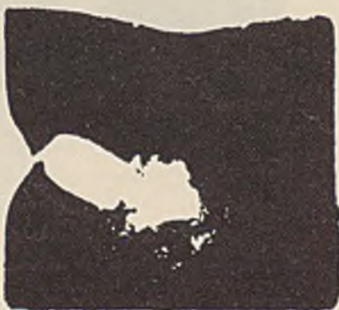
FIG. 8.—Ingot 455 (12% Si). Solidified under 200 lb./in. 2 Pressure.
