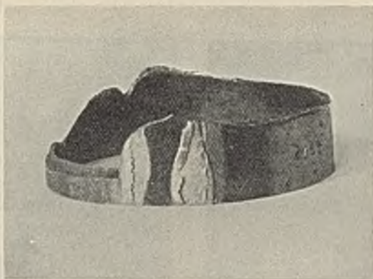
FIG. 2.—Axle-Tube A. Showing Transverse Fatigue Fracture and Longitudinal Intercrystalline Crack.
