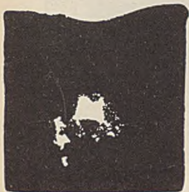
FIG. 7.—Ingot 447 (12% Si). Solidified under 50 lb./in. 2 Pressure.
