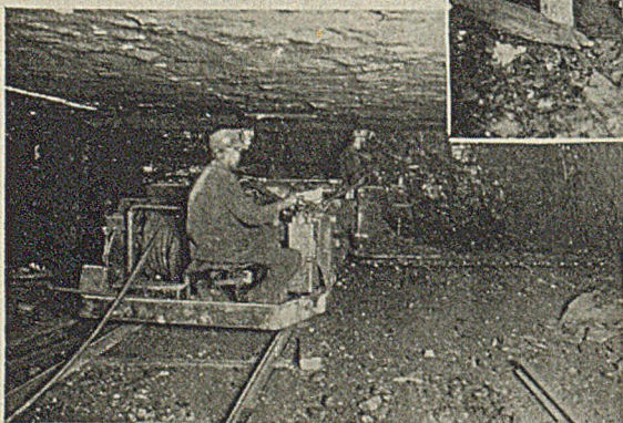
Bottom-Cutting a 26-Ft. Room
