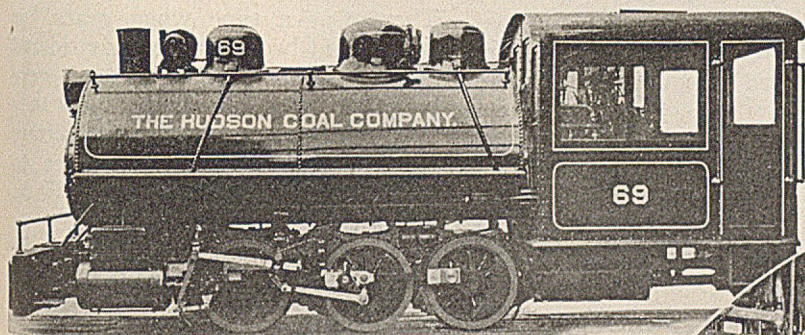
Equipped With Walschert Valve Gear to Reduce Maintenance
