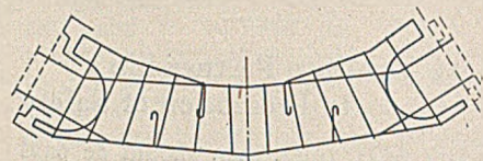
Fig. 3—Section of Kabelac Lining Showing Reinforcement
