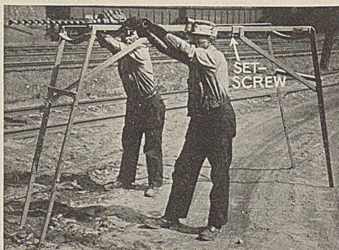
Portable Drill Mounting for Hand Feed
