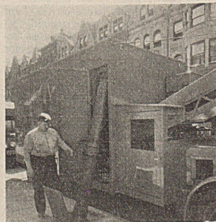
Pneumatic Ash-Conveyor System: Truck With Pipe Placed in Sidewalk Opening
