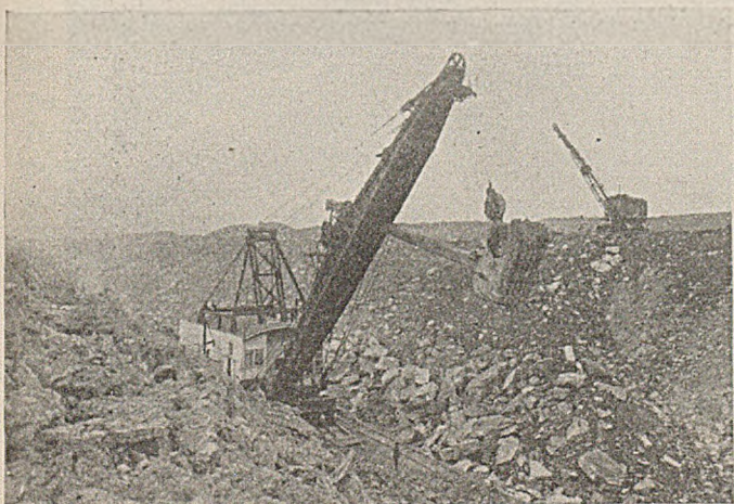
Fig. 1—The Stripped Area Is Nearly Flat Where Dragline Has Operated
