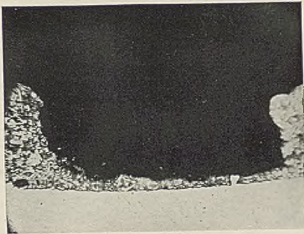
FIG. 6.—Cross-Section of a Fatigued White Metal Coating, Showing Separation during Service of a Cracked Section. \times 50 .
