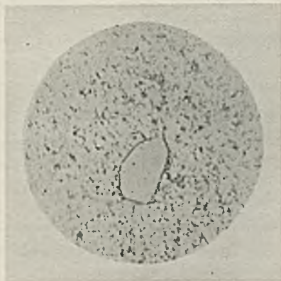
FIG. 6.—0.01% Copper. Annealed at 220° C. for 15 Days and Quenched. \times 500 .
