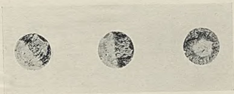
FIG. 7.—Typical Fractures of Fatigue Test-Pieces. \times 2
