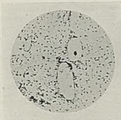
FIG. 5.—0.11% Copper. Annealed at 220° C. for 17 Days and Quenched. \times 500 .
