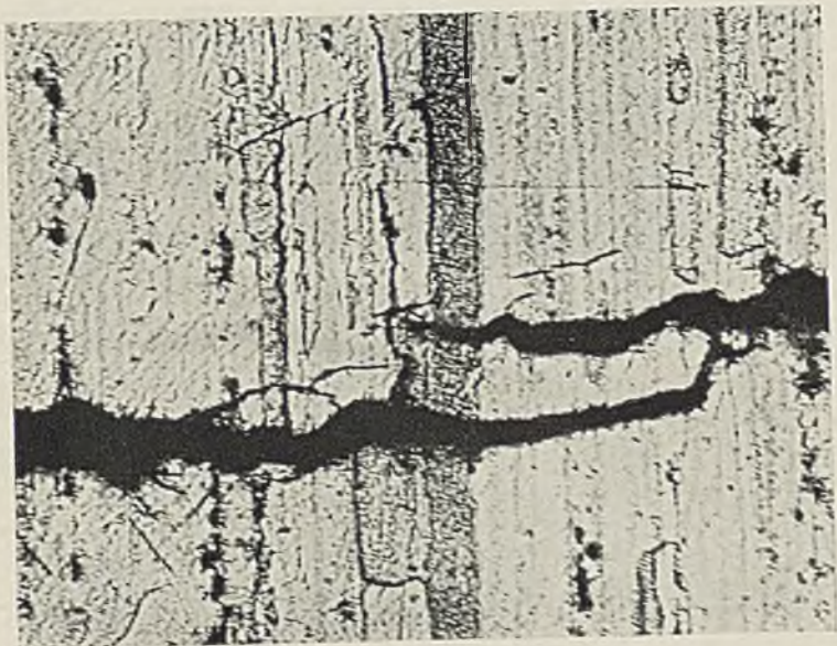
FIG. 6.—Section from Broken Fatigue Test-Piece, Etched. \times 200
