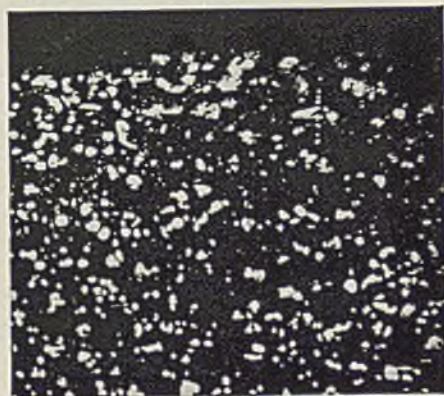
FIG. 5.—P 3. 91.89% Sn, 5.12% Sb, 2.98% Cu. Cold-rolled; section. \times 1000 .
