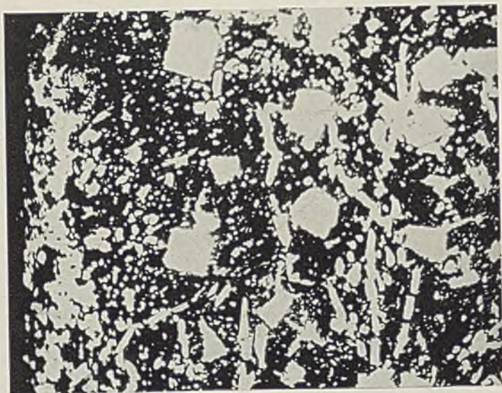
FIG. 25.—Alloy II after Pounding. \times 250 .
