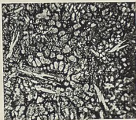
FIG. 2.—P 3. 91.89% Sn, 5.12% Sb, 2.98% Cu. As cast. \times 750 .
