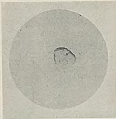
FIG. 3.—0.005% Nickel. Annealed at 228° C. for 7 days and Quenched. \times 1000 .
