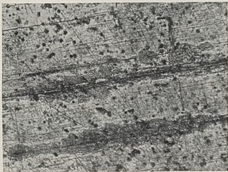
FIG. 44.—Corrosion-Fatigue of a Single Crystal of Aluminium, showing Selective Corrosive Attack and Initiation of Cracks along Slip Bands. \times 100 .
