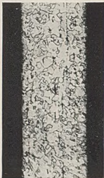
FIG. 4.—Etched Section of Wire shown in Fig. 3 (left). \times 200 .
