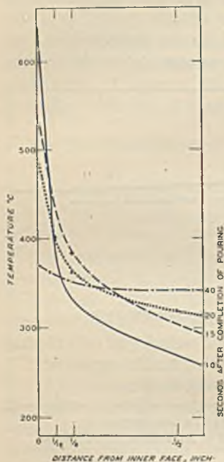
FIG. 12.—Temperature Gradients in Mild Steel Mould Wall.
