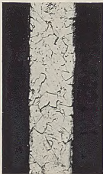
FIG. 14.—Refined Nickel annealed at 720° C. \times 500.
