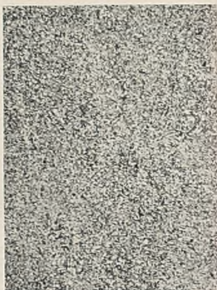
FIG. 7.—Annealed \frac{1}{2} hr. at 610° C. \times 100 .
