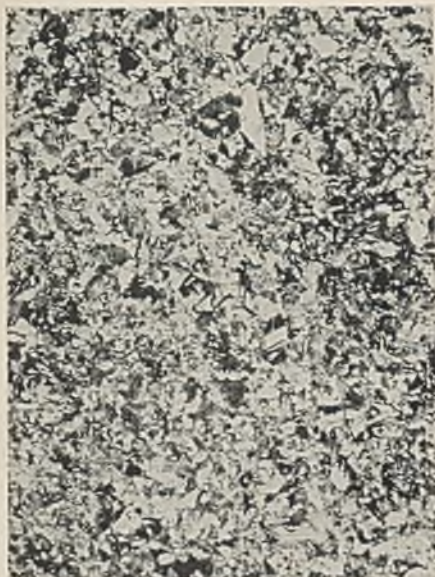
FIG. 2.—Annealed \frac{1}{2} hr. at 400° C. \times 100 .
