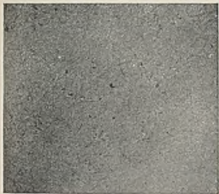
FIG. 4.—19 per cent. Tin. Quenched from 182° C. \times 40 .
