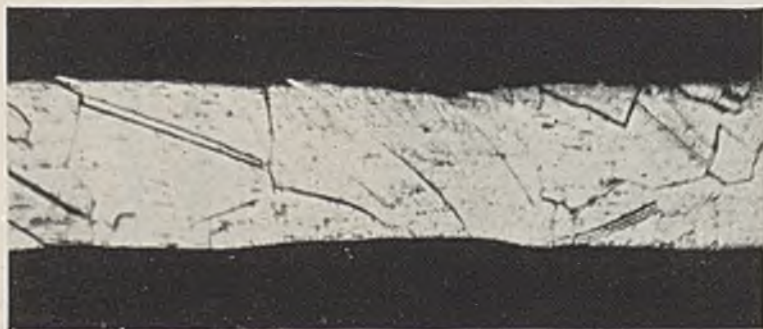
FIG. 6.—Etched Section of Tensile Specimen showing necking in a single crystal. \times 200 .
