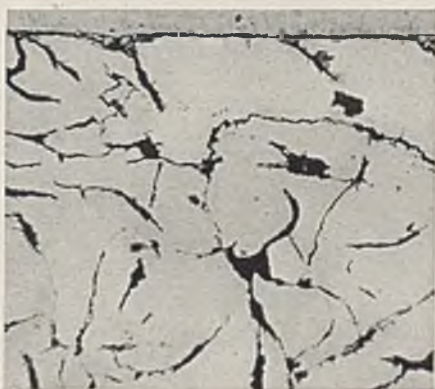
FIG. 7.—Edge of Cylinder shown in Fig. 6, Showing Decarburization of Pearlite. \times 250 .
