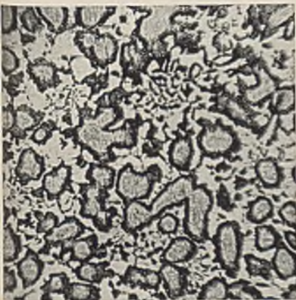
FIG. 3.—50% quaternary alloy. "Soaked" at 905° C. Near top. Silver: 48.0%. \times 80 .
