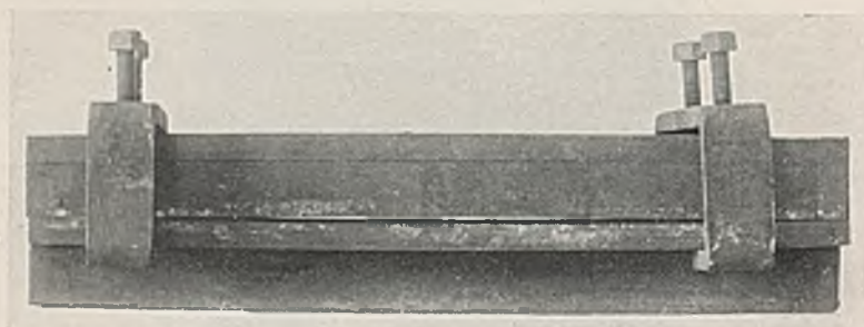
FIG. 10.—Mild Steel Ingot Mould after 6 Heats. \times \frac{1}{6} .
