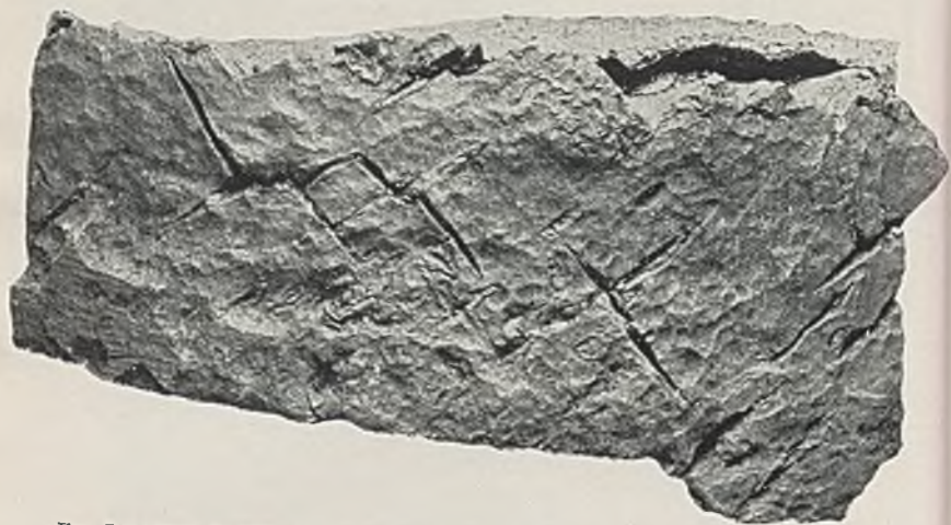
FIG. 7.—Ship's Tail Shaft (9 in. diam.) Fractured in Service under Corrosion-Fatigue.
