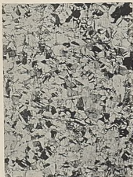
FIG. 4.—Annealed \frac{1}{2} hr. at 500° C. \times 100 .
