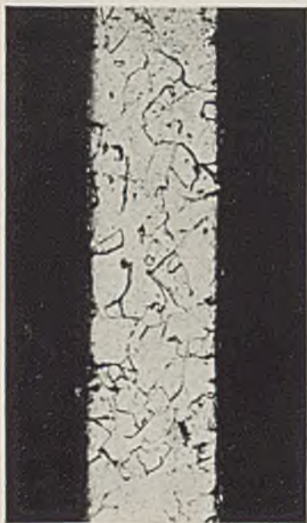
FIG. 12.—Nickel + Iron annealed at 620° C. \times 500.
