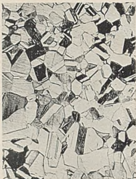
FIG. 6.—Annealed \frac{1}{2} hr. at 610° C. \times 100 .
