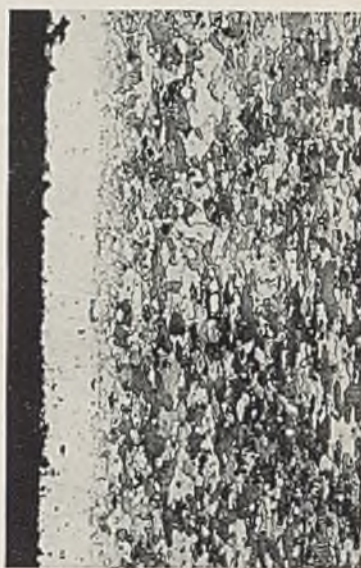
FIG. 11.—2.0 mm. Strip after 3 months' Exposure. \times 100 .
