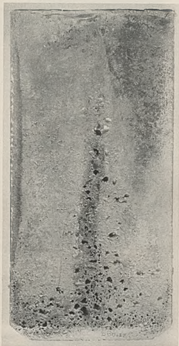
FIG. 1.—70:30 Brass Ingot Cast in Grey Iron Mould, Showing Extensive "Blowing" Defects. \times \frac{1}{2} .
