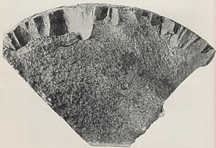
FIG. 8.—Fractured Surface of the Shaft shown in Fig. 7.
