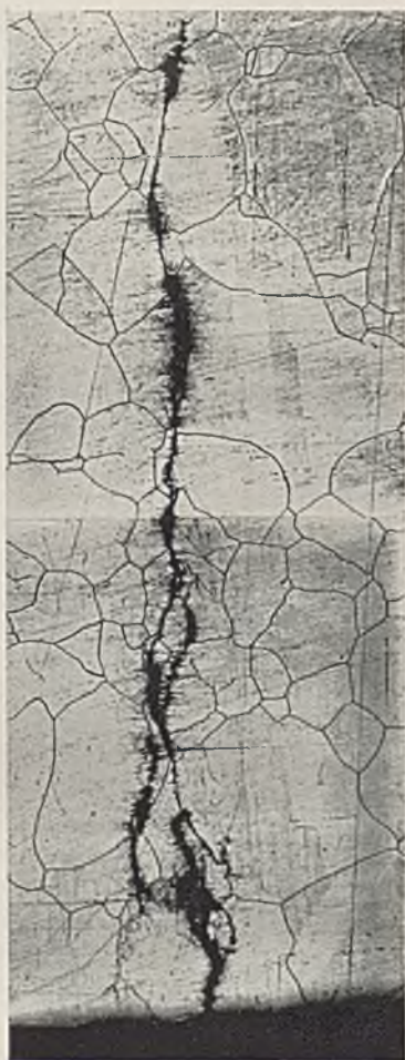
FIG. 38.—Laboratory Specimen of 18:8:1 Cr-Ni-W Austenitic Steel. Failed after 11,167,000 Cycles of \pm 8.3 tons/in. 2 while Subjected to a Drip of Ammonium Sulphate Liquor (50° C.) throughout Test. \times 100 .
