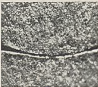
FIG. 3.—Second draught: load required to draw through die 230 pounds. Diameter after drawing 0.0978 inch. Magnification 17.7 diameters.
