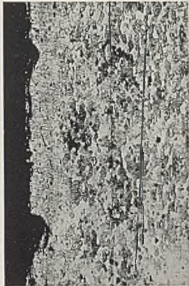
Fig. 15.—2.0 mm. Strip after 18 months' Exposure. \times 100 .
