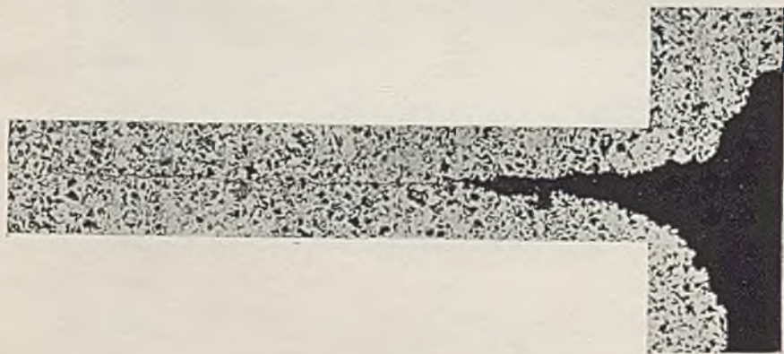
FIG. 4.—Corrosion Pit and Fatigue Crack in Piston Rod (Water-Cooled).
