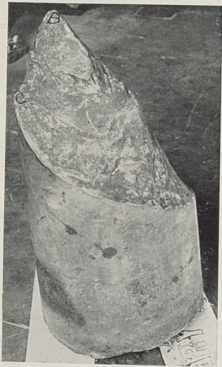
FIG. 11.—Shaft Failure in Tapered Portion of Tail Shaft Originating at Keyway in Boss.
