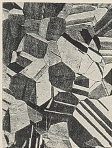
FIG. 8.—Annealed \frac{1}{2} hr. at 700° C. \times 100 .
