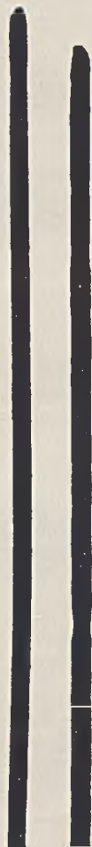
FIG. 3.—Left : Fine-grained Wire showing general elongation. Right : Coarse-grained Wire showing local elongation. \times 20 .
