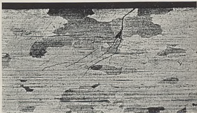
FIG. 39.—Transcrystalline Corrosion-Fatigue (Sea-Water) Fracture of Aluminium (99% Pure). \times 20 .
