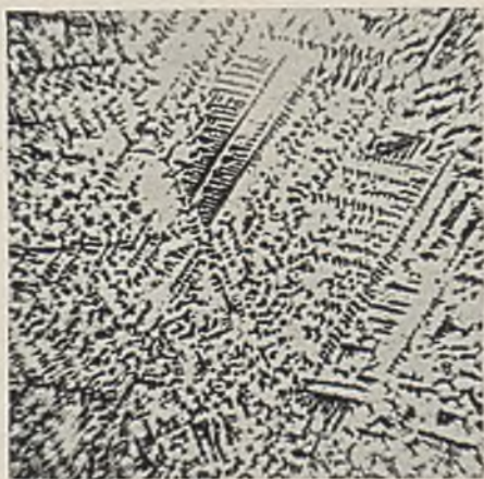
FIG. 7.—50% Ag-Cu. As Fig. 5. Near bottom. Silver: 54.0%. \times 40 .
