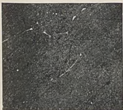
FIG. 6.—19 per cent. Tin. Quenched from 191° C. \times 100 .
