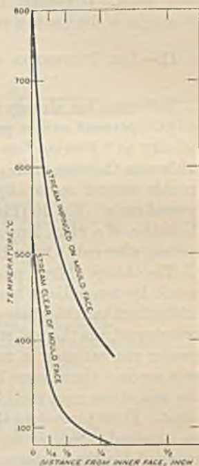
FIG. 9.—Maximum Temperature Gradient in Cast-Iron Mould Wall.
