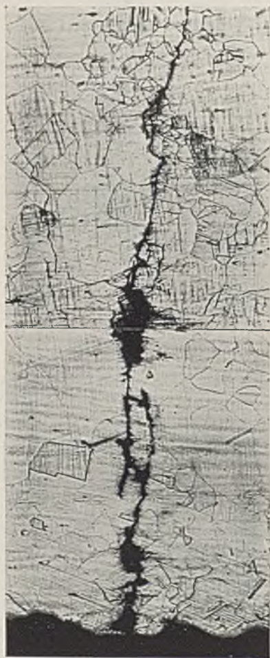
FIG. 37.—Steel Tube (18:8:1 Cr-Ni-W) Failed in Service, by Corrosion-Fatigue, while Conveying a High-Velocity Stream of Boiling Ammonium Sulphate Liquor: the Tube was in a State of Vibration. \times 100 .
