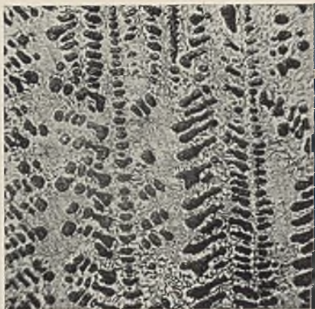
FIG. 2.—50% Ag-Cu. As Fig. 1. Near bottom. Silver: 57.0%. \times 80 .
