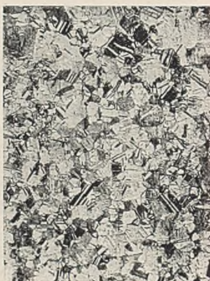
FIG. 9.—Annealed \frac{1}{2} hr. at 700° C. \times 100 .
