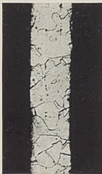
FIG. 13.—Nickel + Iron annealed at 720° C. \times 500.
