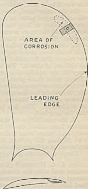
FIG. A. Note.—The small hatched portion indicates the position from which the specimen was taken.
