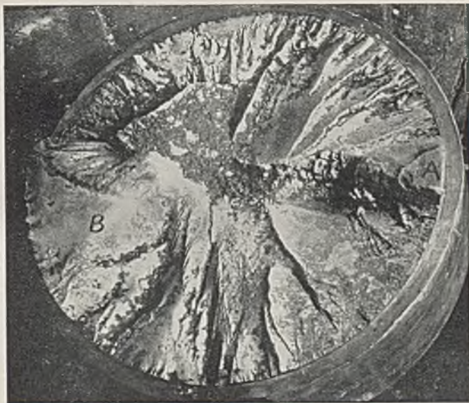
FIG. 6.—Marine Propeller Shaft (14 in. diam.) Failed by Corrosion-Fatigue due to Leakage of Water between Propeller Boss and Shaft Liner. Service 15 months.
