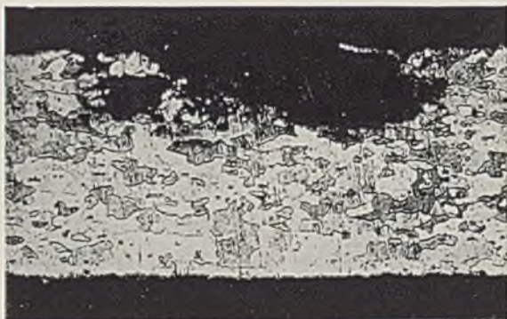
FIG. 17.—0.5 mm. Strip after 24 months' Exposure. Series II. \times 100 .
