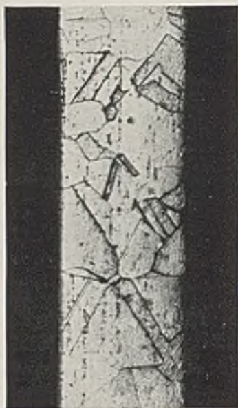
FIG. 5.—Etched Section of Wire shown in Fig. 3 (right). \times 200 .
