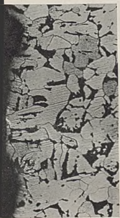
FIG. 32.—Fracture of Mild Steel Specimen after 441,000 Cycles of \pm 16.2 tons/in. 2 while Exposed to a Drip of Tidal River Water. \times 300 .
