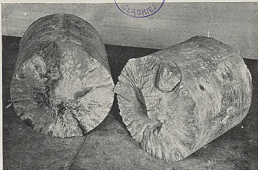
FIG. 9.—Fracture of Marine Propeller Shaft (16 in. diam.) Occurring between Two Sections of the Brass Protective Sleeve. Service 3½ years.
