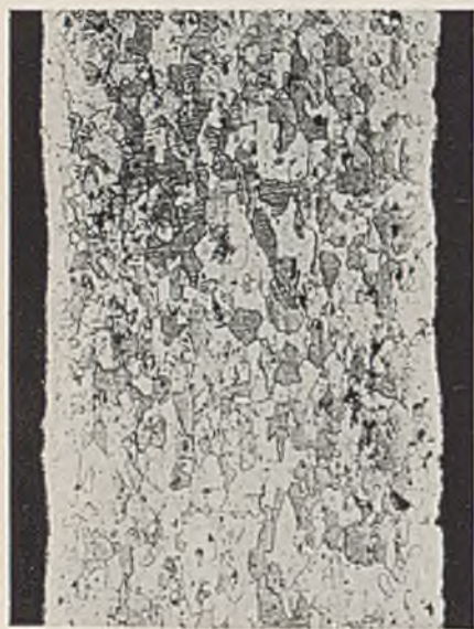
FIG. 8.—0.5 mm. Strip after 3 months' Exposure. \times 100 .
