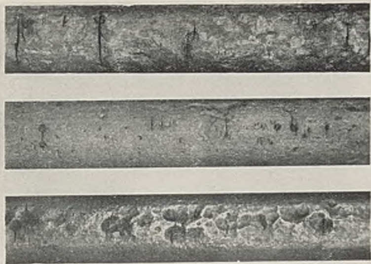
FIG. 17.—Corrosion-Fatigue Failures of Pump Rods in Various Stages of Development.
