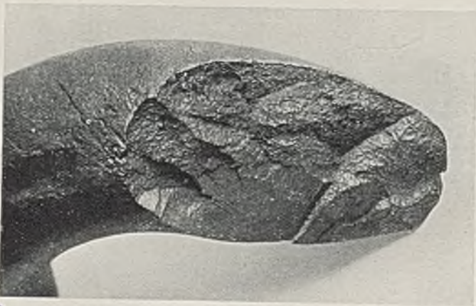
FIG. 15.—Corrosion-Fatigue Failure of a Railway Helical Spring.
