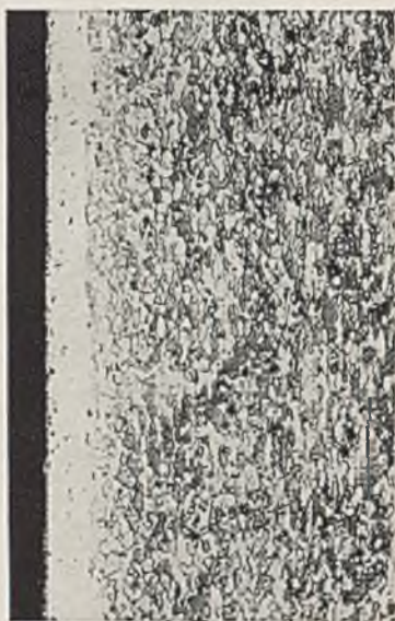
FIG. 10.—1.5 mm. Strip after 3 months' Exposure. \times 100 .
