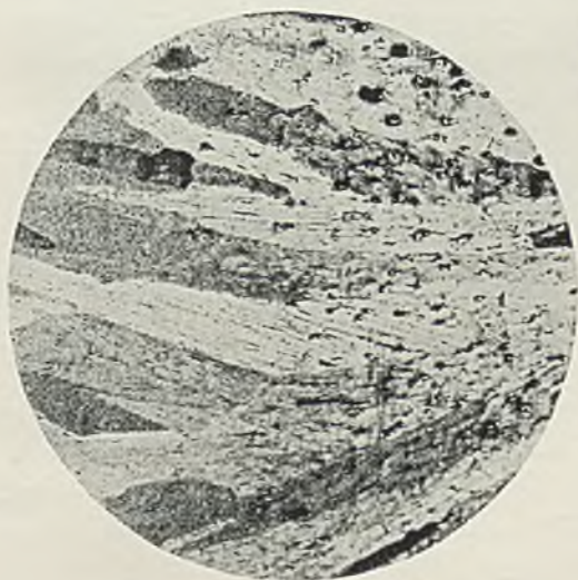
FIG. 3.—Transition from Sound to Porous Regions in Copper Ingot. \times 5 .
