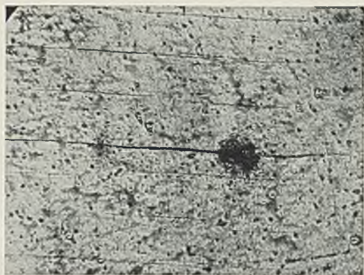
FIG. 7.—Preferential corrosion on slip band (after second test). (\lambda = 259.5^\circ, d = -9.4.) \times 100
