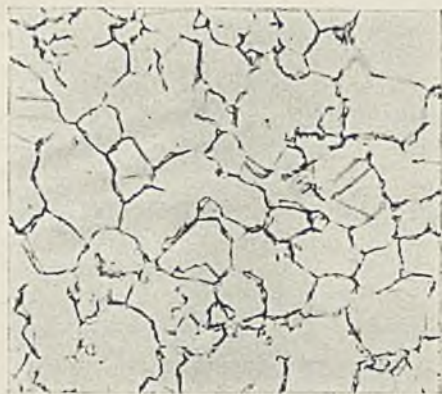
FIG. 1.—Alloy 27 (Nickel 6%, Aluminium 1.5%). Quenched from 900° C. Diamond Pyramid Hardness 75. \times 250 .
