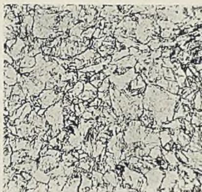
FIG. 2.—As Fig. 1, but Tempered for 2 hours at 500° C. Diamond Pyramid Hardness 187. \times 250 .
