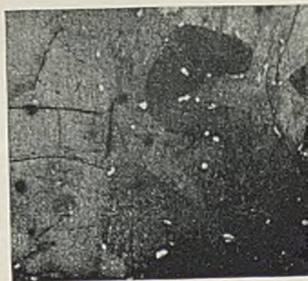
FIG. 8.—Same alloy as Fig. 7. Quenched from 588° C. \times 150. \theta + \eta .
