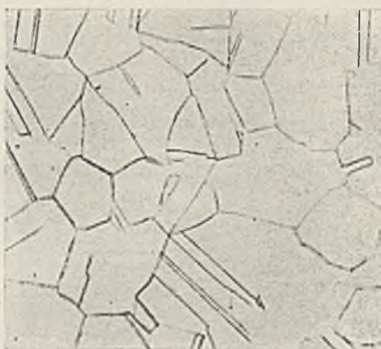
FIG. 6.—Alloy 8 (Nickel 6.6%, Aluminium 3.3%). Quenched from 900° C. and Tempered.
