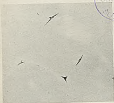
FIG. 3.—52.68% Copper. Quenched from 570° C. \times 150. \theta + traces of liquid.
