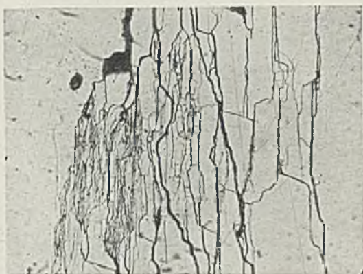
FIG. 11.—Branching of crack 1 (on cross-section). \times 330 .
