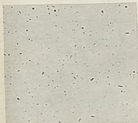
FIG. 5.—52.68% Copper. Quenched from 403° C. \times 150. \theta + \kappa (black).
