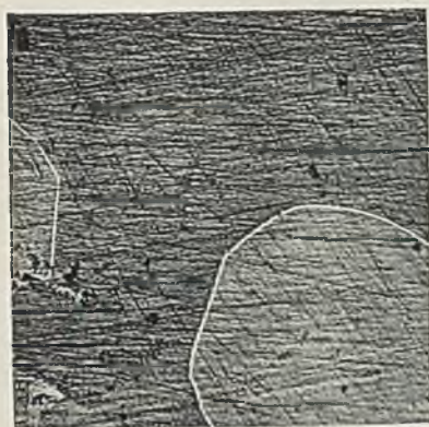
FIG. 4.—9.95 per cent. Aluminium. Slowly Cooled. \gamma (dark) and \beta' (white) at the Boundary. \times 50 .
