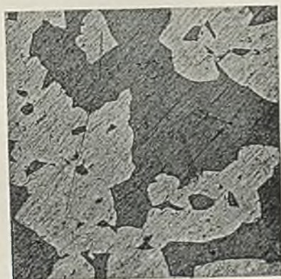
FIG. 5.—7.48 per cent. Aluminium. Quenched at 600^{\circ} C. \alpha (grey) and \gamma (dark). \times 50 .
