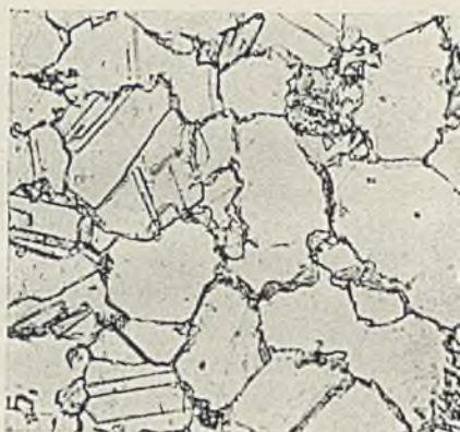
FIG. 4.—Alloy 26 (Nickel 10%, Aluminium 2.5%). Quenched from 900° C. Diamond Pyramid Hardness 94. \times 250 .
