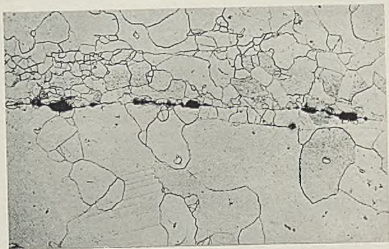
FIG. 2.—Lead Pipe Showing Defects due to Annular Lamination. Etched with Ammonium Molybdate and followed by Glycerol Reagent. \times 50 .
