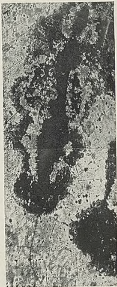
FIG. 14.—End of crack 2 (after fourth test). ( \lambda = 84^\circ , d = 0.3 ) \times 100 . Reduced by \frac{1}{4} in reproduction.
