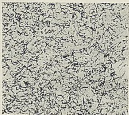
FIG. 3.—Alloy 27 (Nickel 6%, Aluminium 1.5%). Hard-Rolled. Tempered at 500° C. for 30 minutes. Diamond Pyramid Hardness 190. \times 250 .
