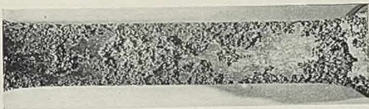
FIG. 1.—Untreated Elektron AZM Alloy Test-Bar after Immersion in Sea-water. Corrosion Product Removed.
