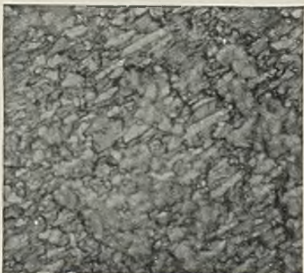
FIG. 14.—Extruded Lead-Tin Eutectic Alloy, Annealed 5 hrs. at 100^{\circ}\text{C} . Strained Rapidly. Unetched. \times 1000 .
