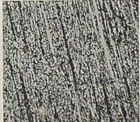
FIG. 6.—Longitudinal Section from Extruded Bismuth-Tin Alloy. Etched with Ferric Chloride. \times 100 .
