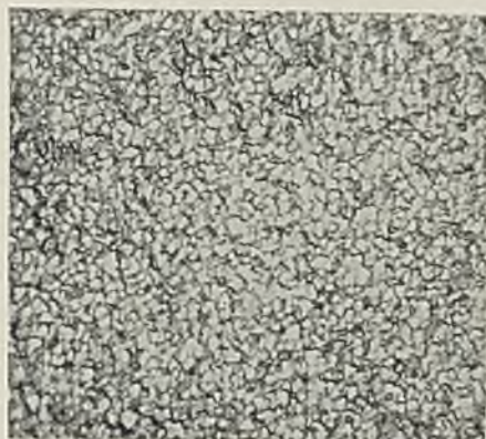
FIG. 9.—Extruded Lead-Tin Eutectic, Aged \frac{1}{2} hr. Structure Developed by Straining. Elongation about 50 per cent. Unetched. \times 1000 .
