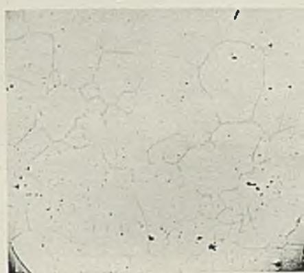
FIG. 10.—45 per cent. Palladium. Quenched from 598° C. \times 50.
