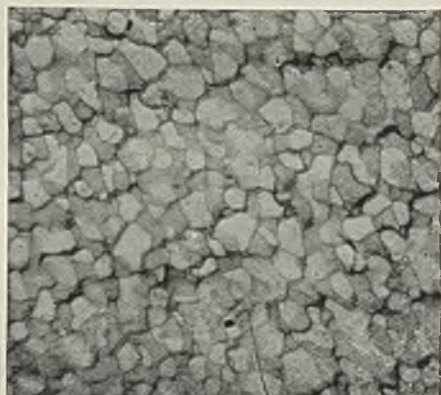
FIG. 12.—As Fig. 9, but Annealed 2 hrs. at 175^{\circ}\text{C} . before Straining. Unetched. \times 1000 .
