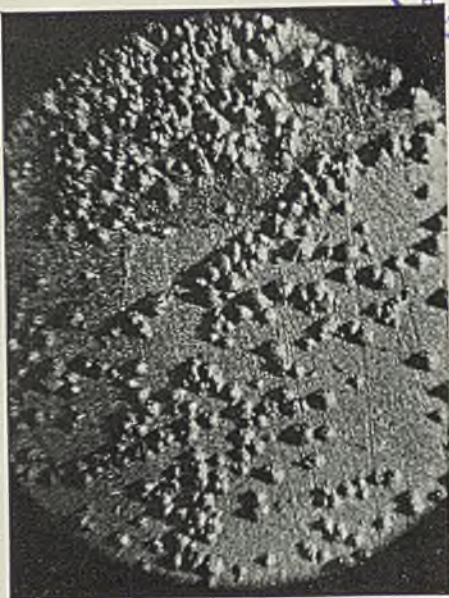
FIG. 1.—Steel Plate Heated for a Short Time at 380° C. in Contact with Zinc. Zinc Plate Removed. \times 28 , Oblique Illumination.
