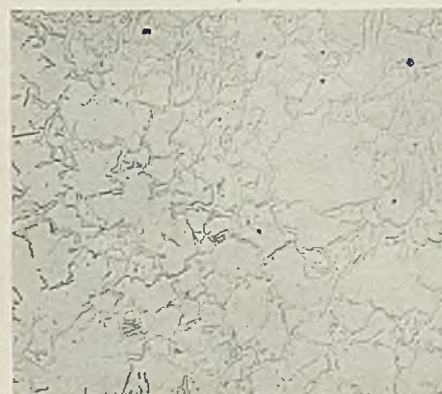
FIG. 7.—42.5 per cent. Palladium. Quenched from 594° C. \times 75.
