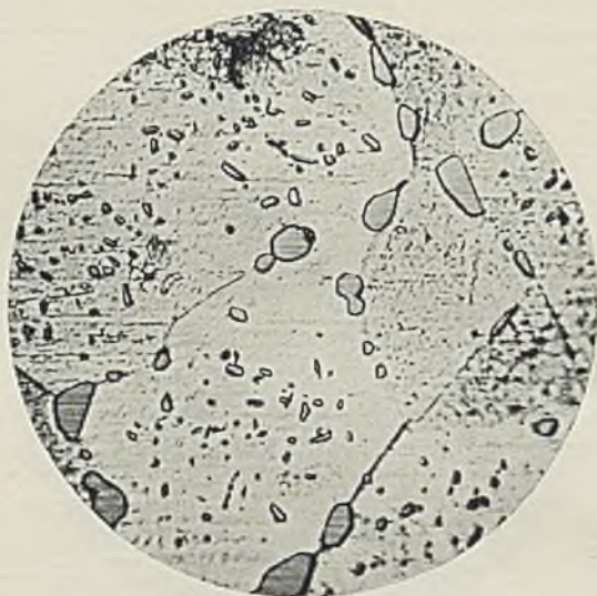
FIG. 17.—Silicon 5.0%, Iron 1%. \alpha + \text{Fe} . \times 500 .
