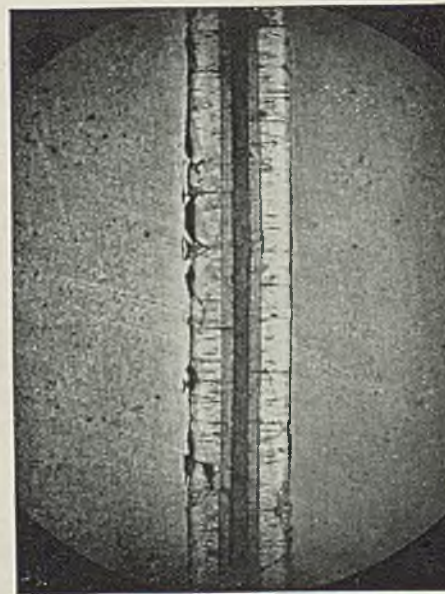
FIG. 4.—Zinc Sheet between Polished Steel Plates. Heated for 71 hrs. at 354° C. \times 21
