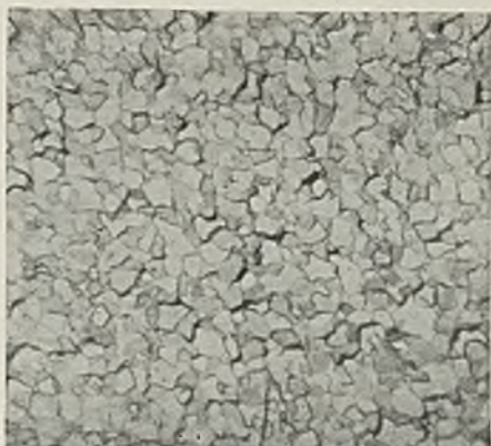
FIG. 11.—As Fig. 9, but Annealed 5 hrs. at 100^{\circ}\text{C} . before Straining. Unetched. \times 1000 .
