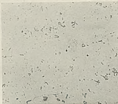
FIG. 12.—50 per cent. Palladium. Quenched from 556° C. \times 75.
