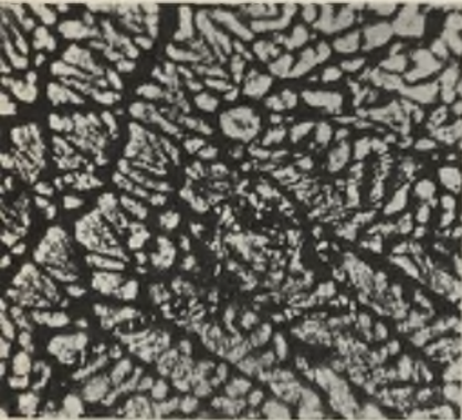
FIG. 1.—P 0. 95.00% Sn, 5.00% Sb. As cast. \times 750 .
