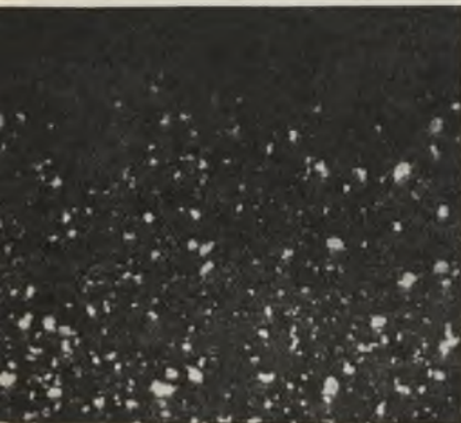
FIG. 4.—P 1. 93.96% Sn, 5.05% Sb, 0.98% Cu. Cold-rolled; section. \times 1000 .
