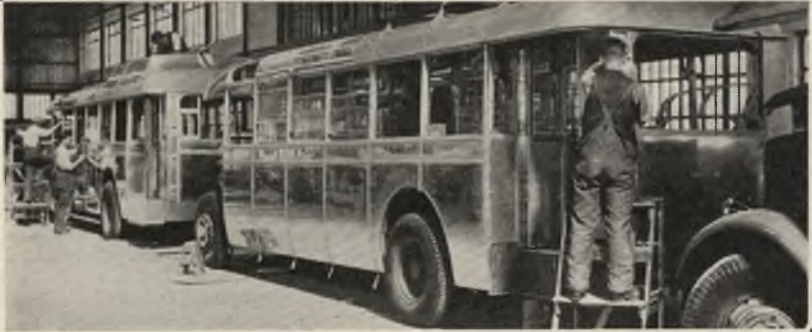
All-Aluminium buses in course of construction at the works of Messrs. H. V. Burlingham Ltd., Blackpool.
